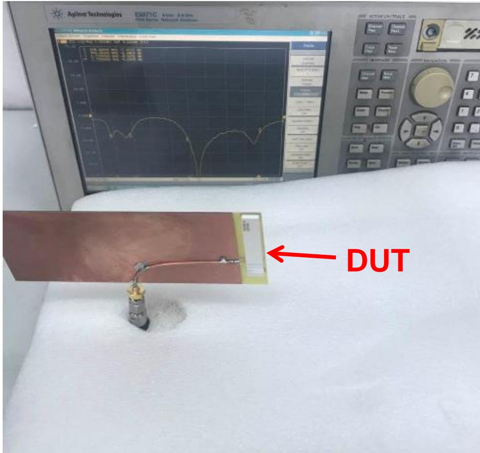
**FIGURE 4.1.2 ANTENNA LOADED ON REFERENCE PCB (130\*48MM) TESTED WITH VNA E5071C**
