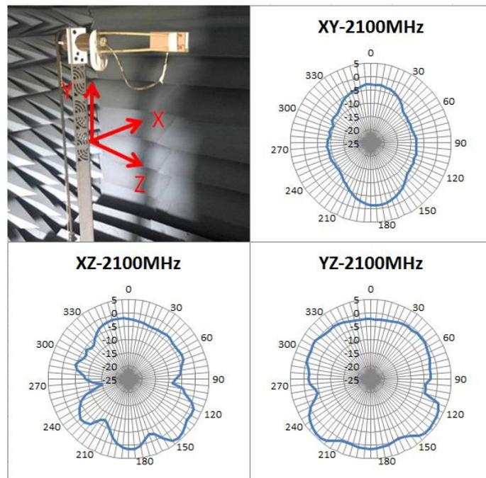
**FIGURE 4.5.4 2D RADIATION PATTERN OF ANTENNA AT 2100MHZ IN FREE SPACE**
