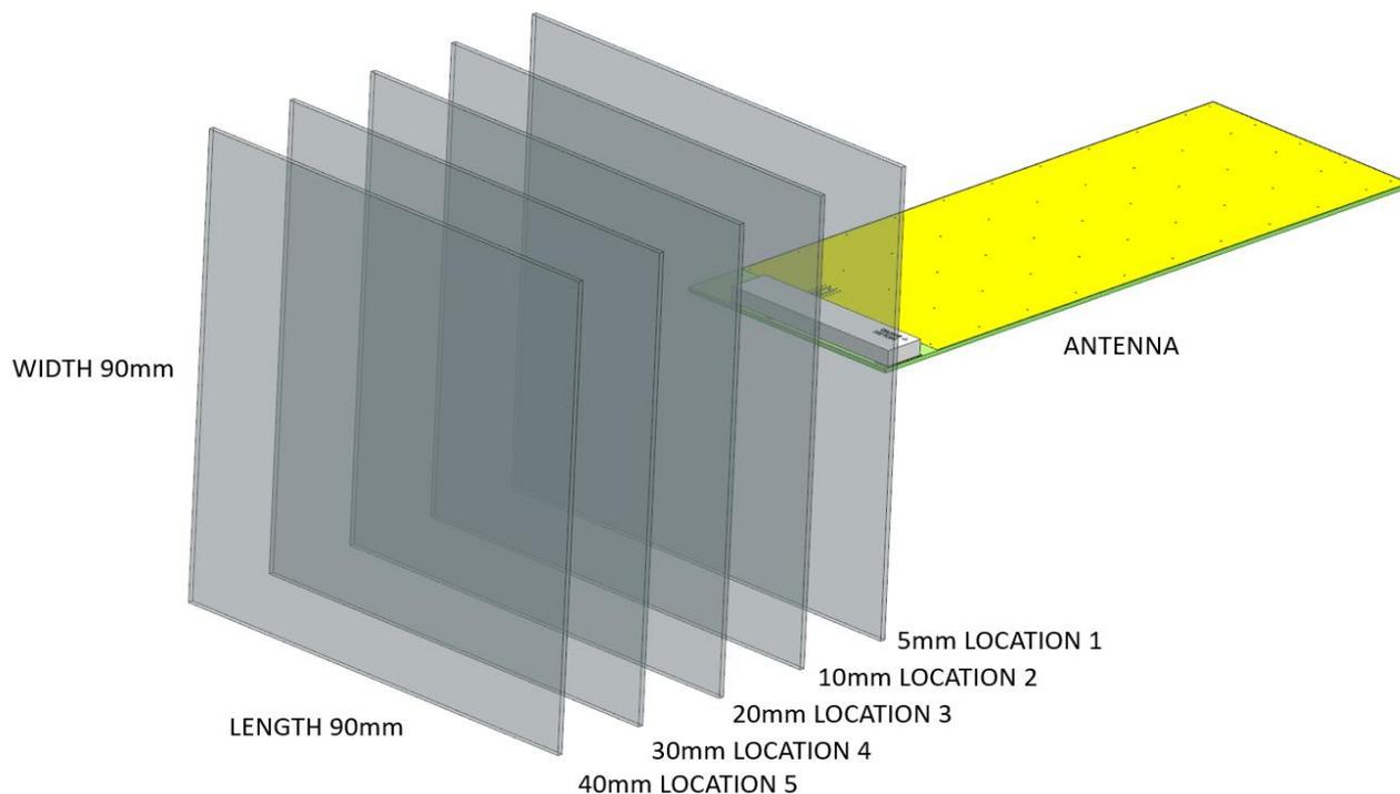
**FIGURE 6.2.1 FIVE LOCATIONS WITH VERTICAL PLANE GROUND**
