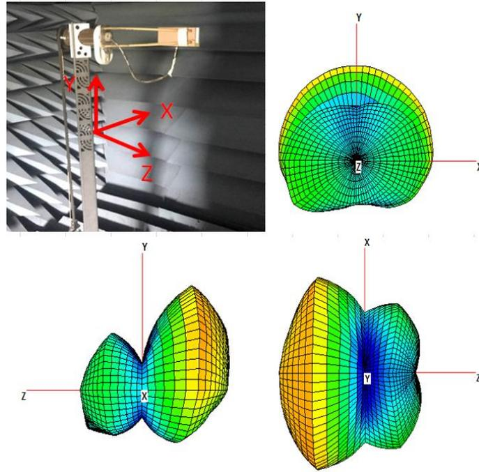
**FIGURE 4.5.9 3D RADIATION PATTERN OF ANTENNA AT 2100MHZ IN FREE SPACE**
