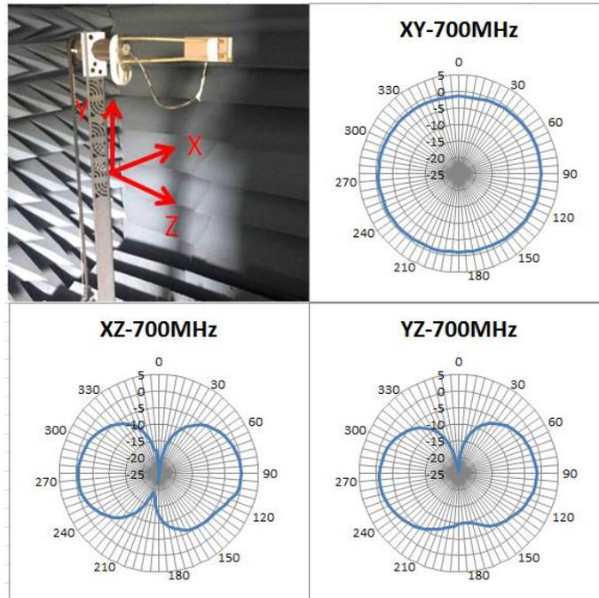
**FIGURE 4.5.1 2D RADIATION PATTERN OF ANTENNA AT 700MHZ IN FREE SPACE**
