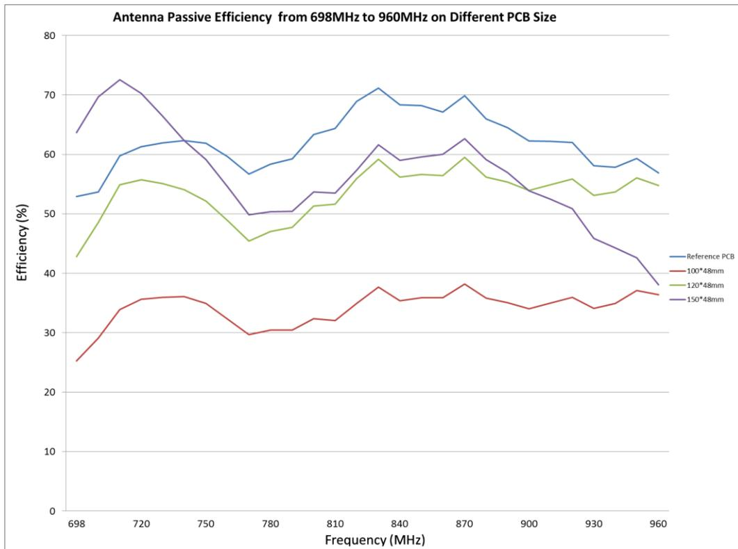
**FIGURE 6.3.4 EFFICIENCY OF ANTENNA FROM 698MHZ TO 960MHZ ON DIFFERENT PCB SIZE**
