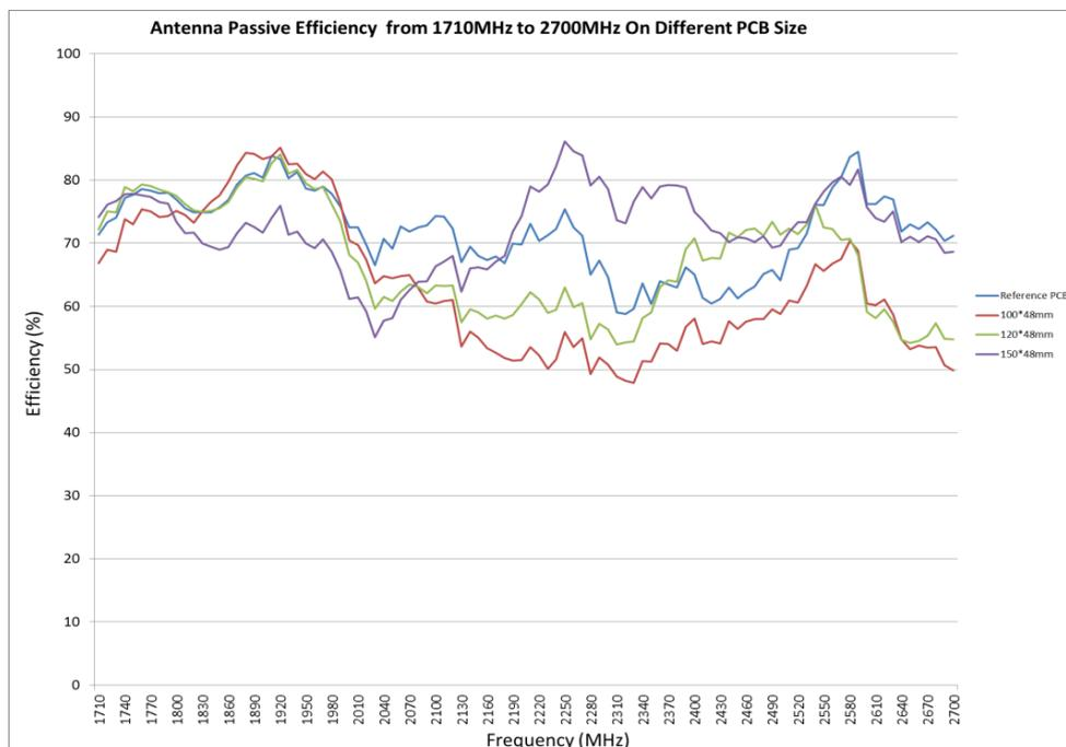
**FIGURE 6.3.5 EFFICIENCY OF ANTENNA FROM 1710MHZ TO 2700MHZ ON DIFFERENT PCB SIZE**
