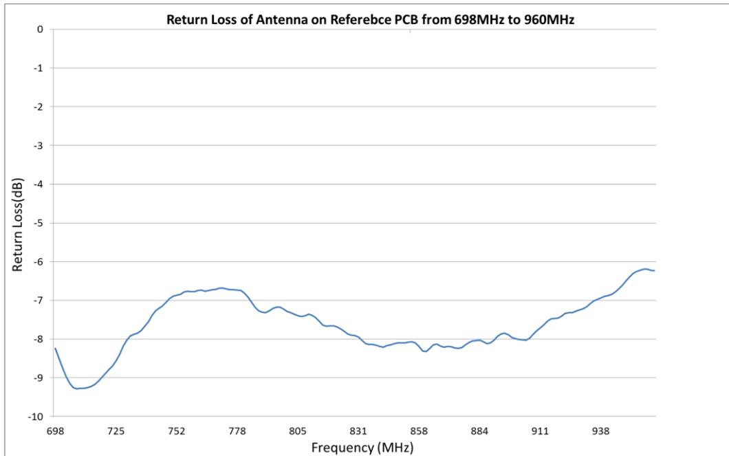
**FIGURE 4.3.1 RETURN LOSS OF ANTENNA FROM 698MHZ TO 960MHZ IN FREE SPACE**
