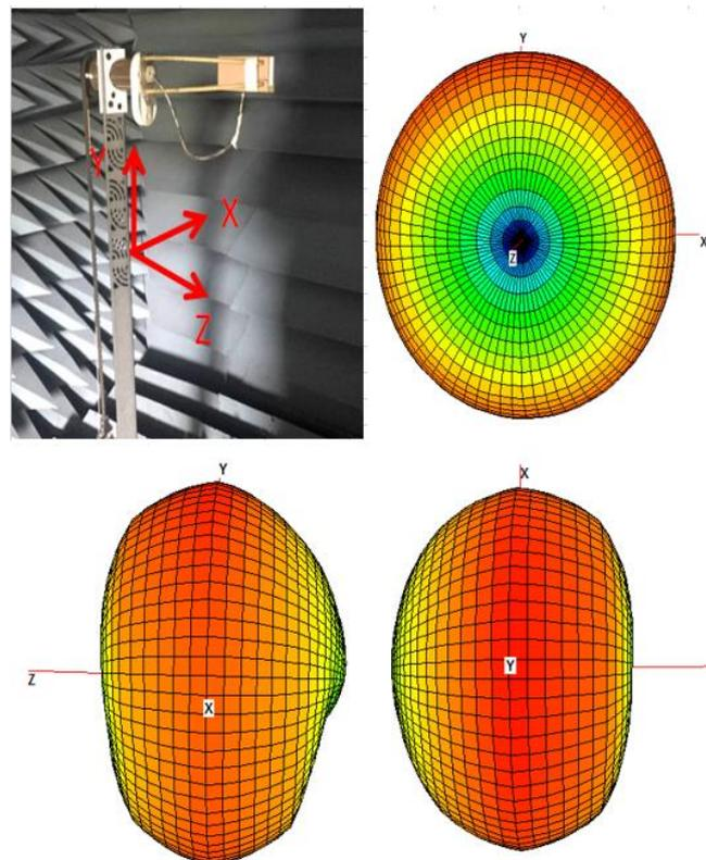
**FIGURE 4.5.6 3D RADIATION PATTERN OF ANTENNA AT 700MHZ IN FREE SPACE**
