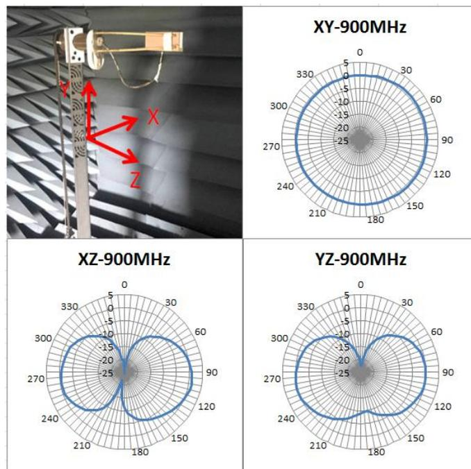
**FIGURE 4.5.2 2D RADIATION PATTERN OF ANTENNA AT 900MHZ IN FREE SPACE**
