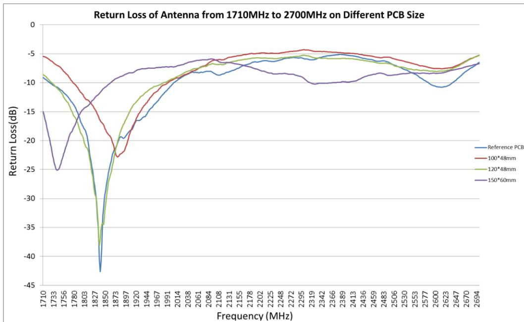
**FIGURE 6.3.3 RETURN LOSS OF ANTENNA FROM 1710MHZ TO 2700MHZ ON DIFFERENT PCB SIZE**
