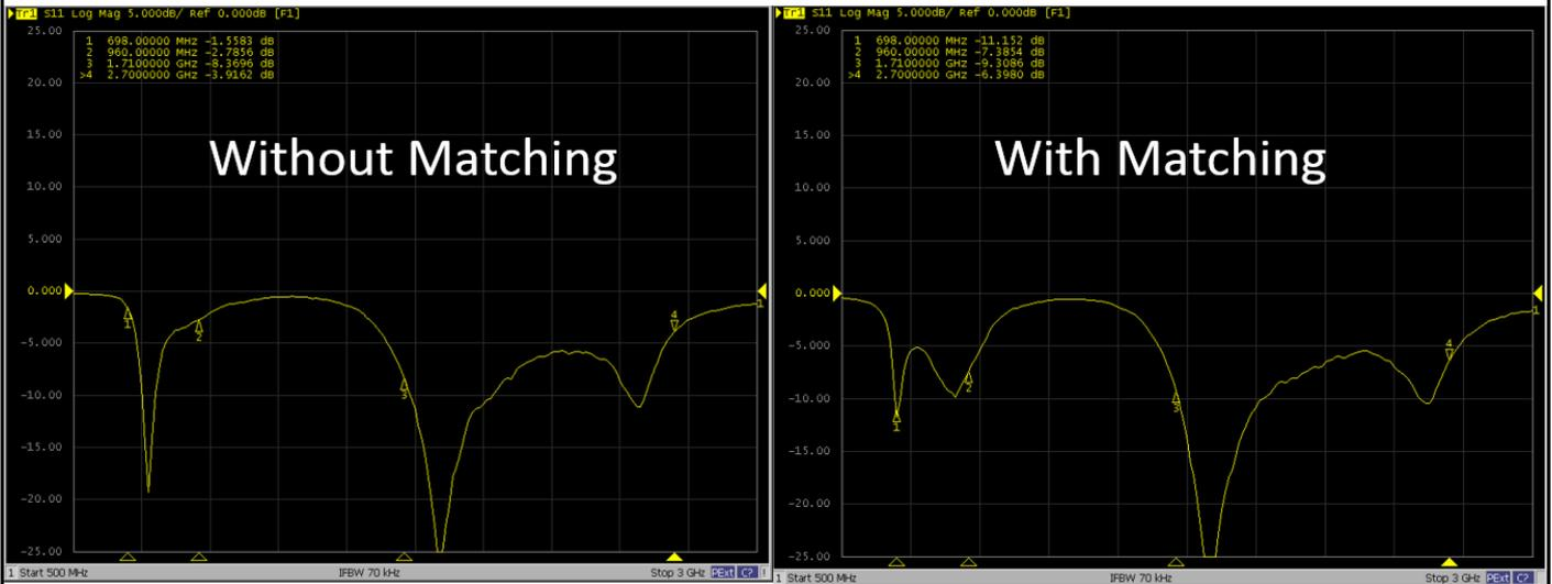
**FIGURE 5.4 RETURN LOSS OF ANTENNA WITHOUT AND WITH MATCHING ON REFERENCE PCB (130\*48MM)**
