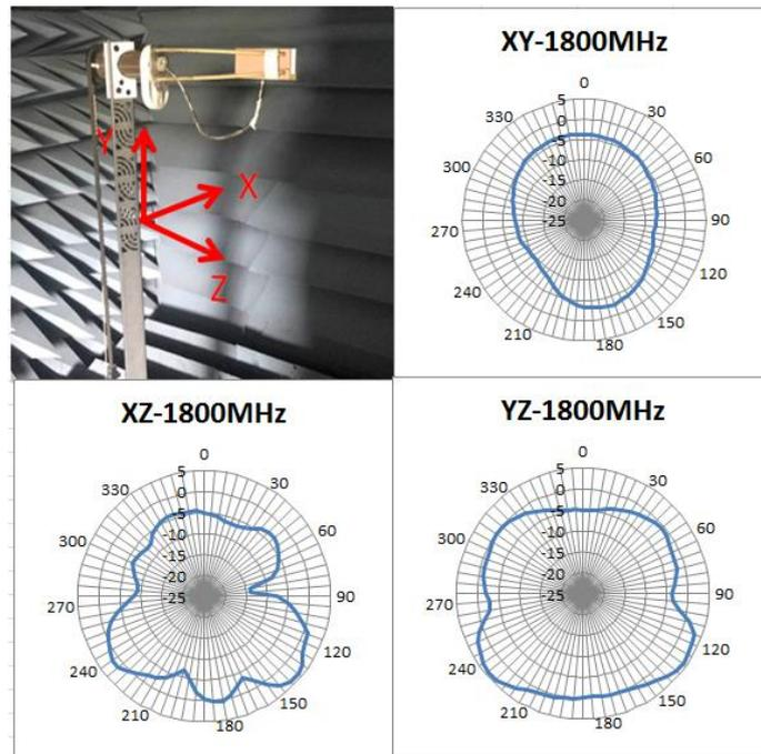
**FIGURE 4.5.3 2D RADIATION PATTERN OF ANTENNA AT 1800MHZ IN FREE SPACE**
