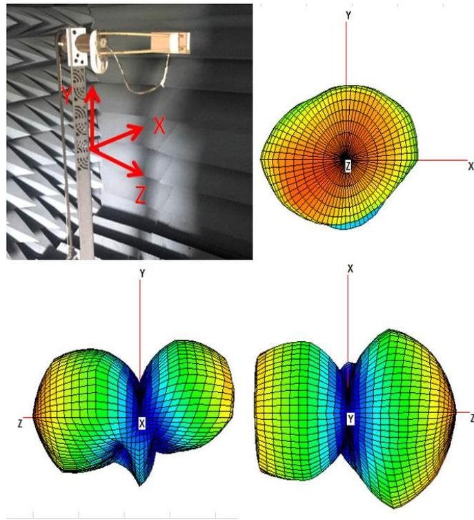
**FIGURE 4.5.10 3D RADIATION PATTERN OF ANTENNA AT 2500MHZ IN FREE SPACE**
