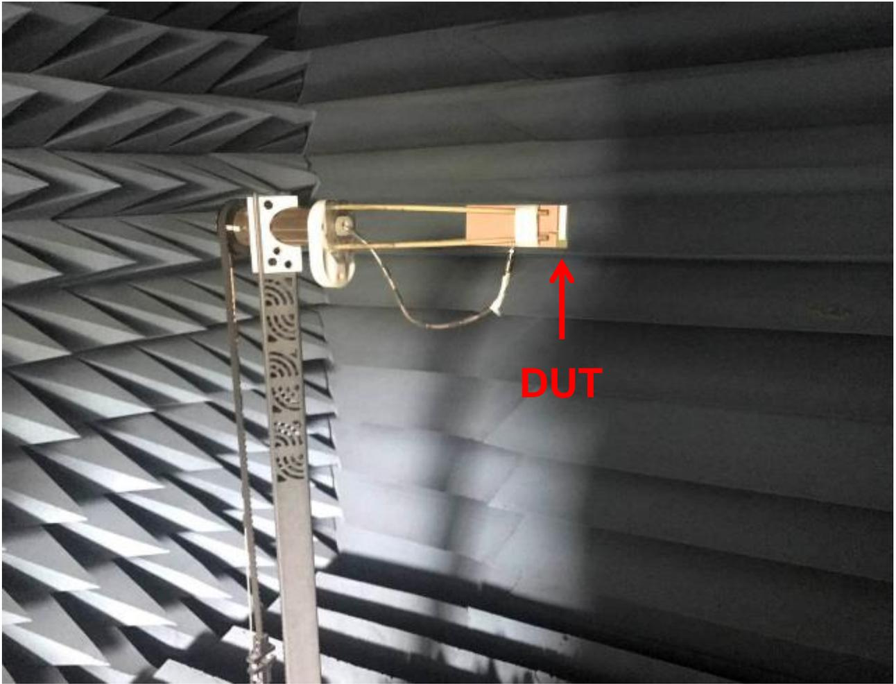
**FIGURE4.1.3 ANTENNA LOADED ON REFERENCE PCB (130\*48MM) TESTED IN OTA CHAMBER**
