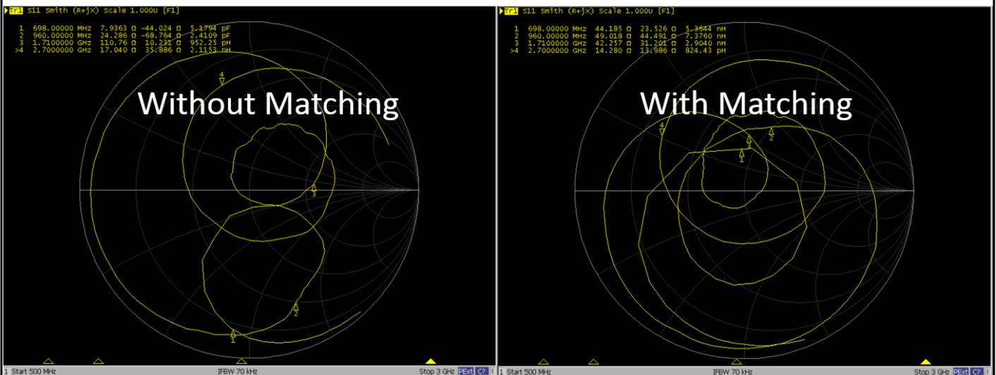
**FIGURE 5.5 SMITH CHART OF ANTENNA WITHOUT AND WITH MATCHING ON REFERENCE PCB (130\*48MM)**
