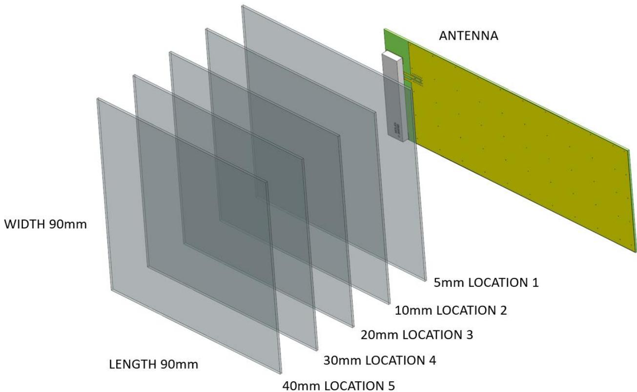
**FIGURE 6.1.1 FIVE LOCATIONS WITH PARALLEL PLANE GROUND**
