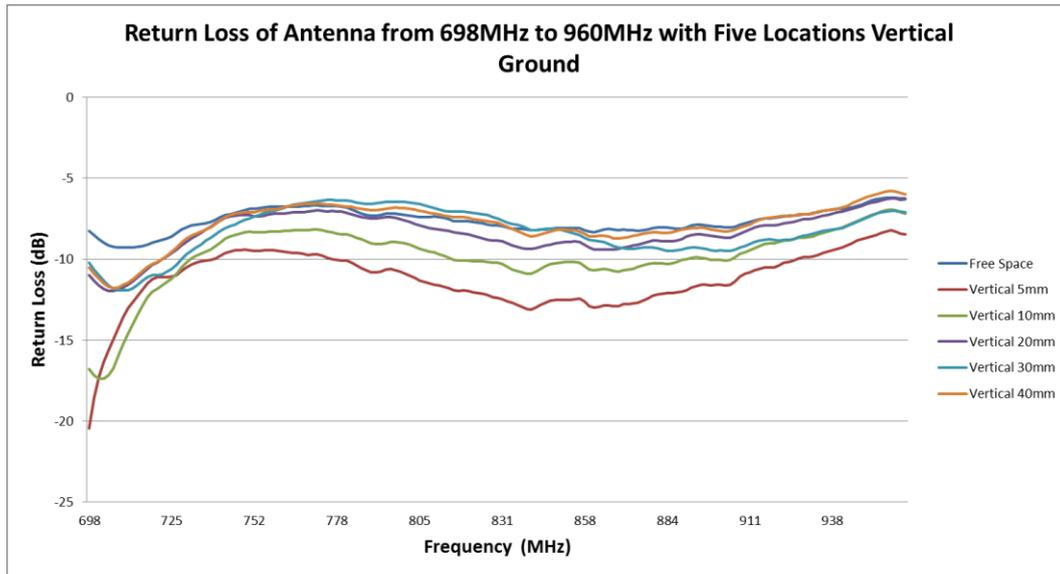
**FIGURE 6.2.2 RETURN LOSS OF ANTENNA FROM 698MHZ TO 960MHZ WITH FIVE LOCATIONS VERTICAL GROUND**
