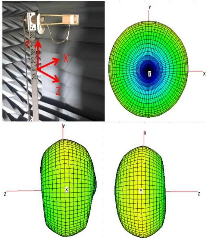
**FIGURE 4.5.7 3D RADIATION PATTERN OF ANTENNA AT 900MHZ IN FREE SPACE**
