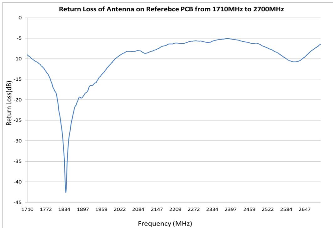
**FIGURE 4.3.2 RETURN LOSS OF ANTENNA FROM 1710MHZ TO 2700MHZ IN FREE SPACE**
