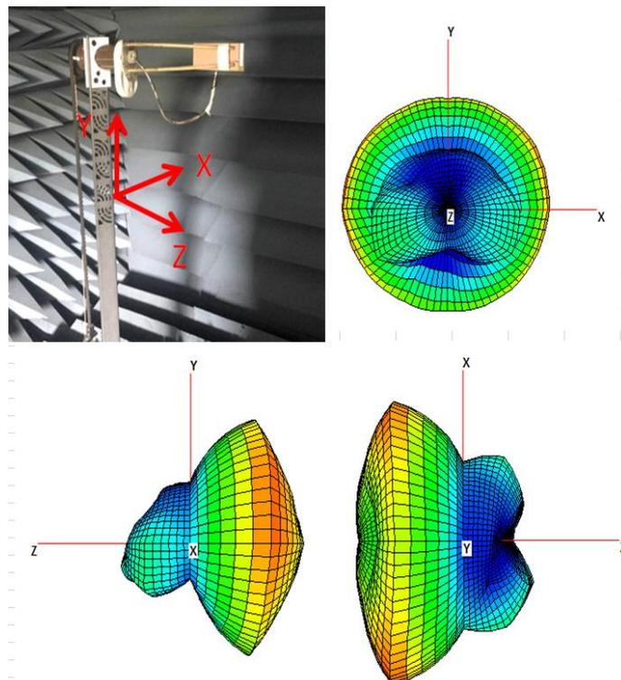
**FIGURE 4.5.8 3D RADIATION PATTERN OF ANTENNA AT 1800MHZ IN FREE SPACE**
