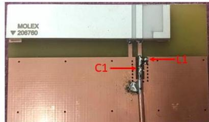
FIGURE 5.3 MATCHING CIRCUIT OF ANTENNA FOR ALL BAND ON REFERENCE PCB (138\*48MM)
