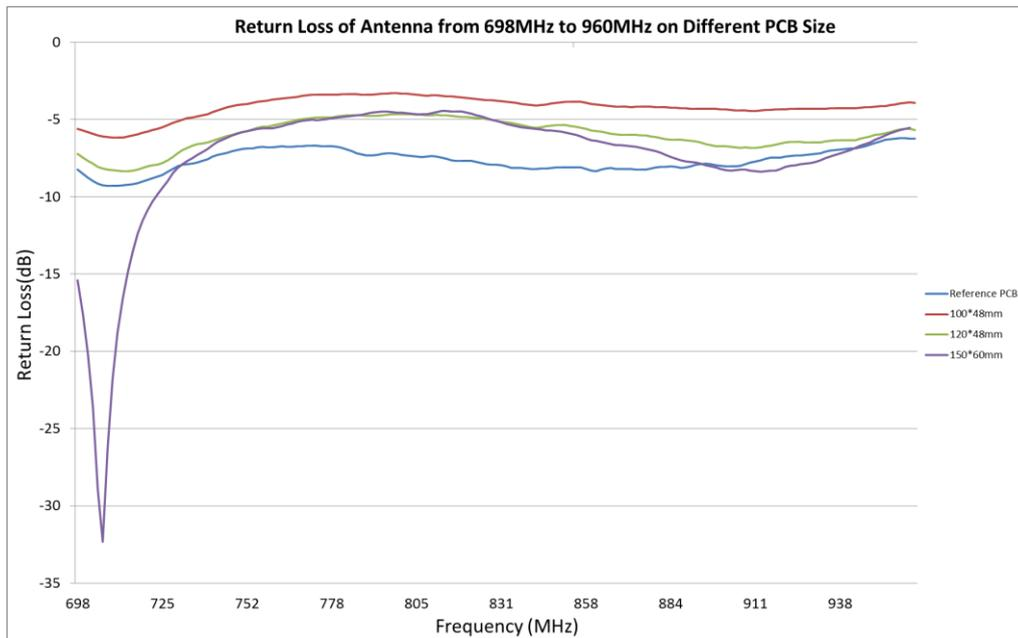
**FIGURE 6.3.2 RETURN LOSS OF ANTENNA FROM 698MHZ TO 960MHZ ON DIFFERENT PCB SIZE**
