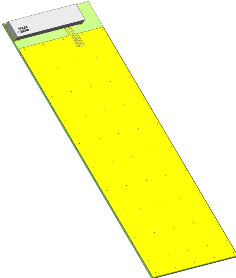
**FIGURE4.1.1 ANTENNA LOADED ON REFERENCE PCB (130\*48MM)**
