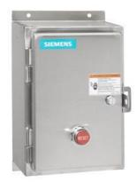
Reversing motor starter, Size 2 1/2, Three phase full voltage, Amb. compensate bimetal OLR, Contactor amp rating 60A, Non-combination type, Encl. type 4X 304 S. Steel, Water/dust tight noncorrosive
