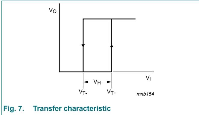
Fig. 7. Transfer characteristic
