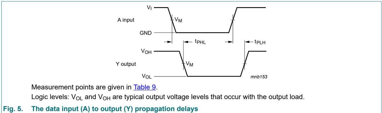
**Fig. 5. The data input (A) to output (Y) propagation delays**
