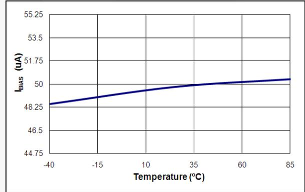
Figure 12. Current Source of IA/IB/IC (I<sub>BIAS</sub>) vs. Temperature
