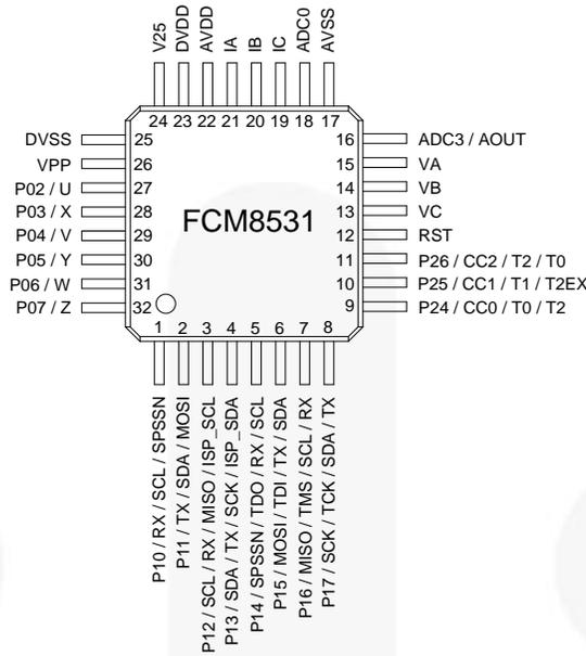
Figure 5. Pin Configuration
