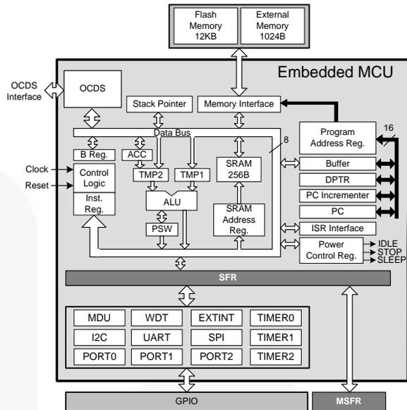
**Figure 20. Embedded MCU Block Diagram**
