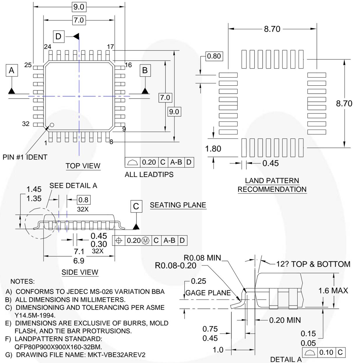
**Figure 28. 32-Low-Profile, Quad, Flat Pack Package (LQFP)**
