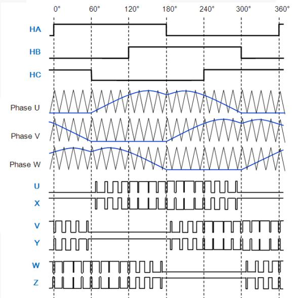
**Figure 18. Default Sine-Wave PWM Output (CW=0)**
