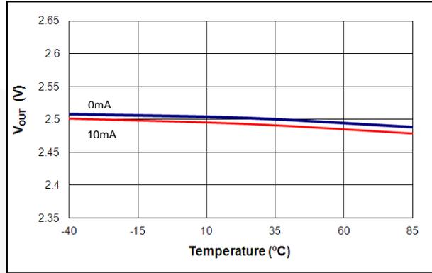
Figure 10. V<sub>25</sub> Output Voltage (V<sub>OUT</sub>) vs. Temperature
