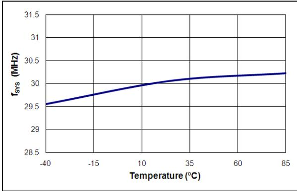
Figure 9. System Frequency (f<sub>sys</sub>) vs. Temperature
