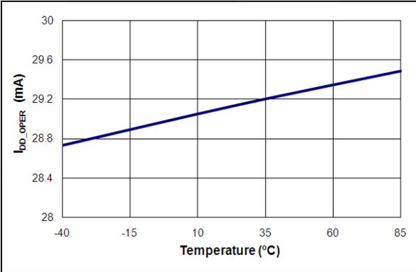
Figure 11. V<sub>DD</sub> Operation Current (I<sub>DD\_OPER</sub>) vs. Temperature
