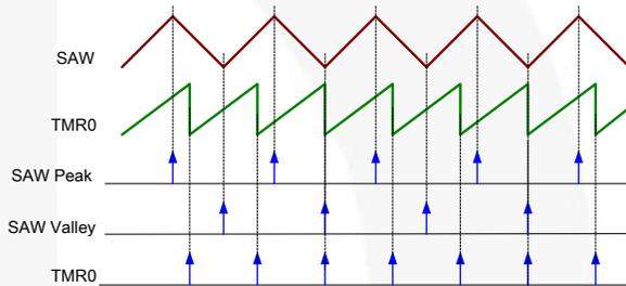
**Figure 25. ADC Trigger Mode**
