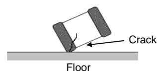
3. When printed circuit boards are piled up or handled, the corner of another printed circuit board should not be allowed to hit the capacitor in order to avoid a crack or other damage to the capacitor.
