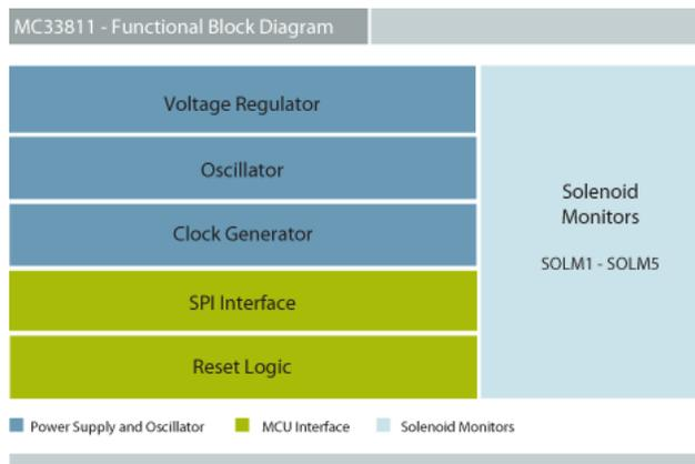
Figure 7. Functional Internal Block Diagram
