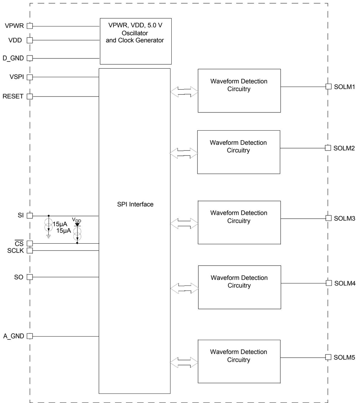
Figure 2. 33811 Simplified Internal Block Diagram
