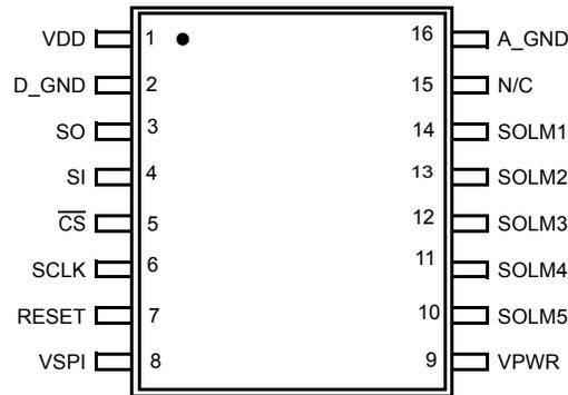
**Figure 3. 33811 Pin Connections**
