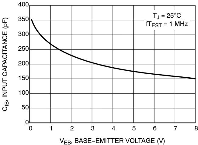
Figure 10. Input Capacitance
