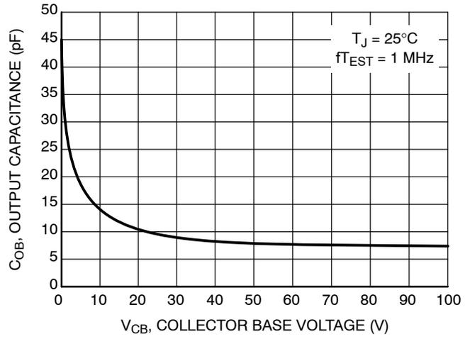
Figure 11. Output Capacitance
