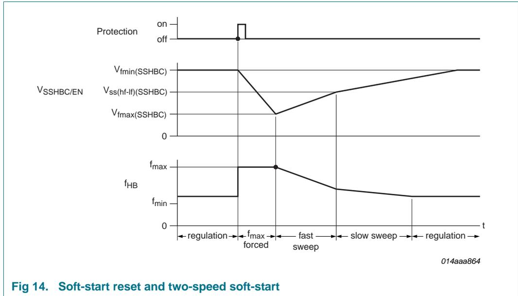
Fig 14. Soft-start reset and two-speed soft-start
