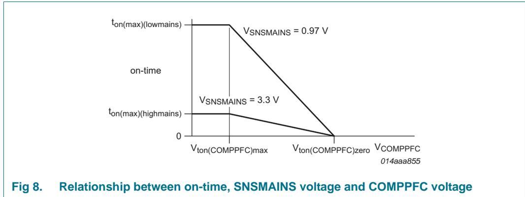
Fig 8. Relationship between on-time, SNSMAINS voltage and COMPPFC voltage
