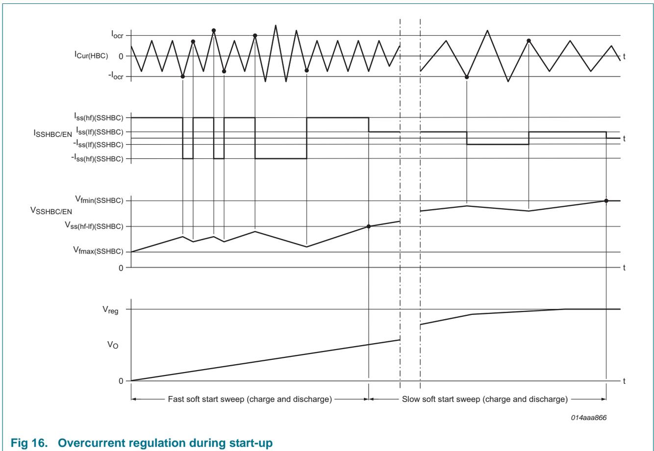
Fig 16. Overcurrent regulation during start-up
