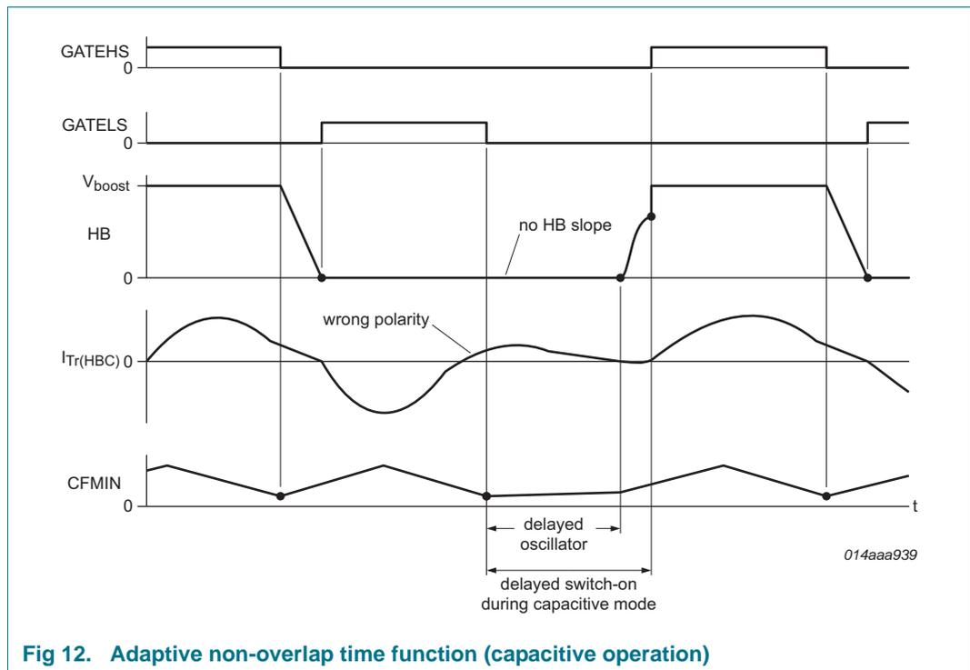
Fig 12. Adaptive non-overlap time function (capacitive operation)
