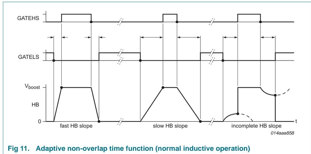
Fig 11. Adaptive non-overlap time function (normal inductive operation)
