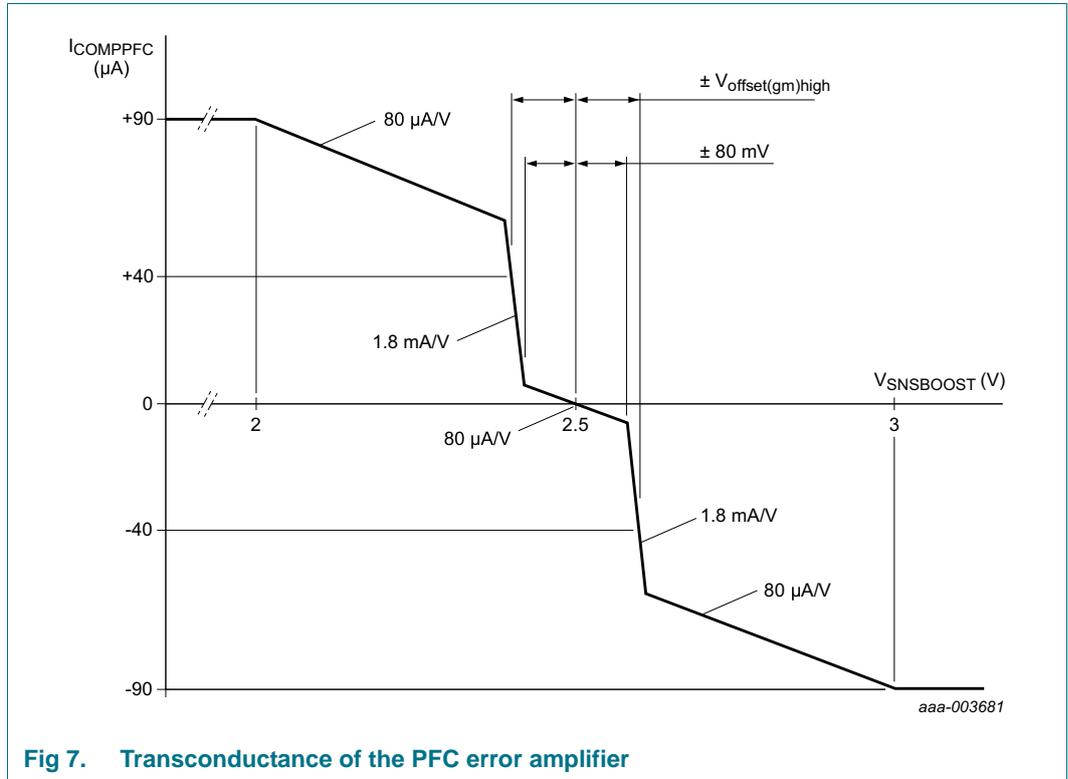
Fig 7. Transconductance of the PFC error amplifier
