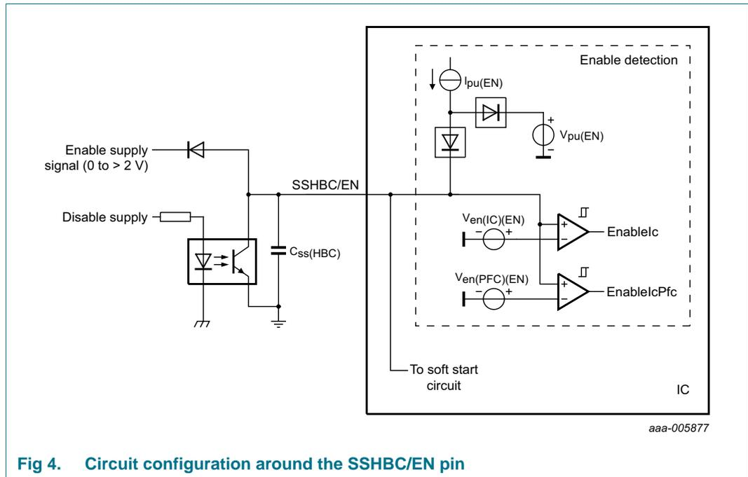
Fig 4. Circuit configuration around the SSHBC/EN pin
