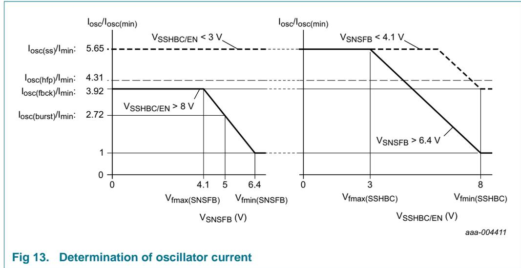
Fig 13. Determination of oscillator current
