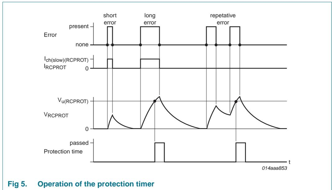
Fig 5. Operation of the protection timer
