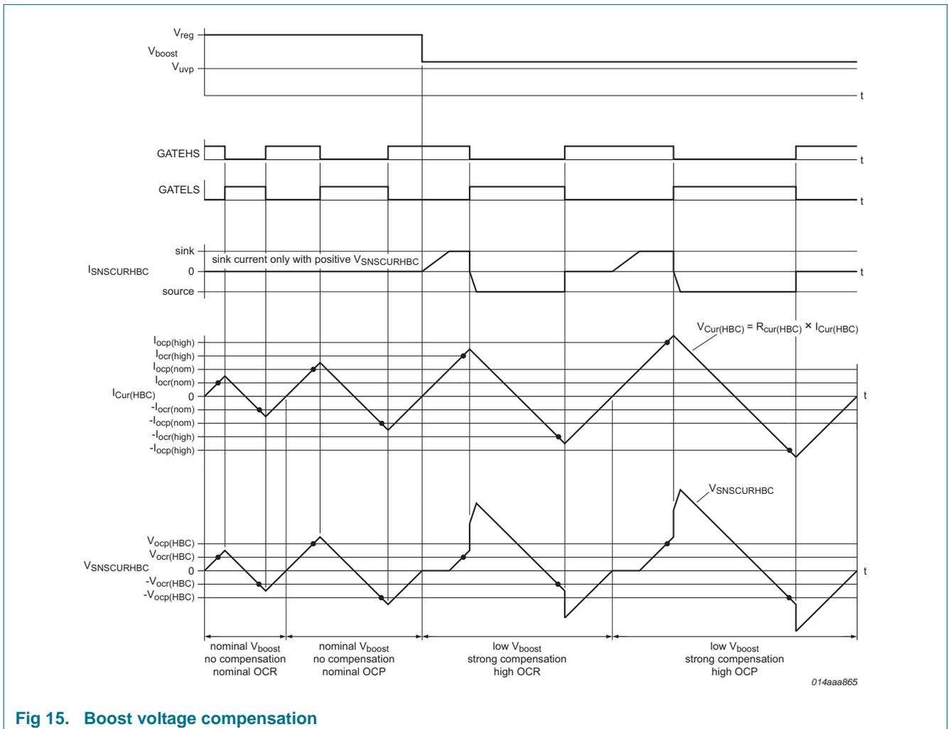
Fig 15. Boost voltage compensation
