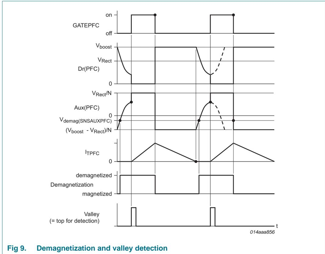
Fig 9. Demagnetization and valley detection
