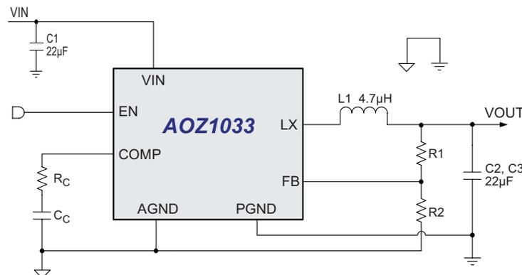
Figure 1. 3.3V 3A Synchronous Buck Regulator
