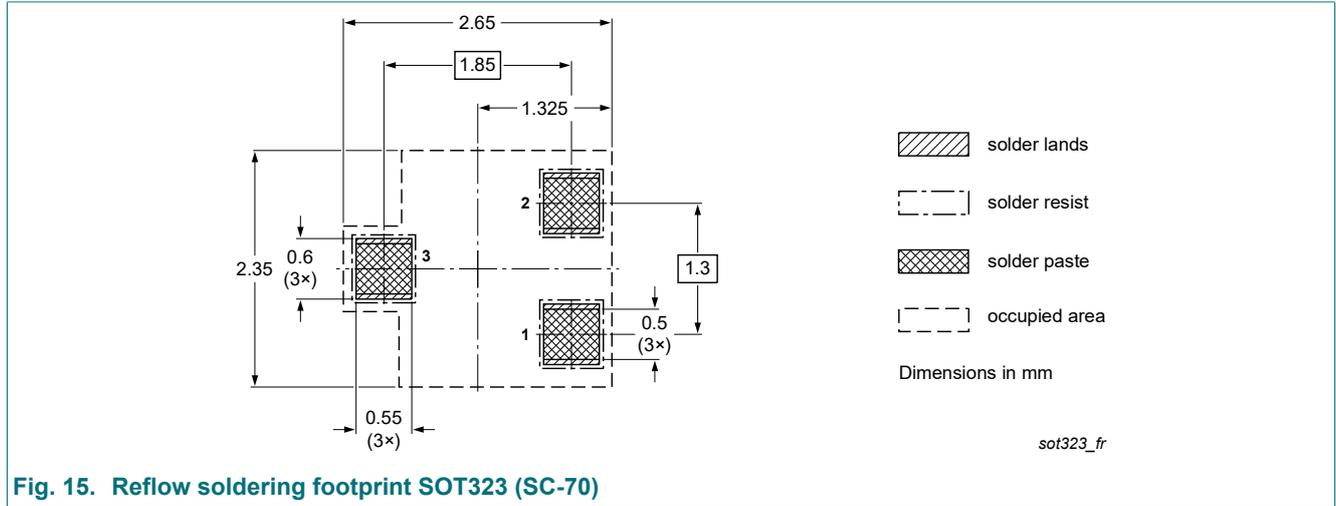
Fig. 15. Reflow soldering footprint SOT323 (SC-70)
