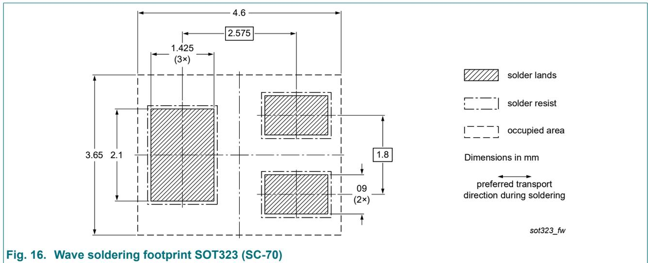
Fig. 16. Wave soldering footprint SOT323 (SC-70)
