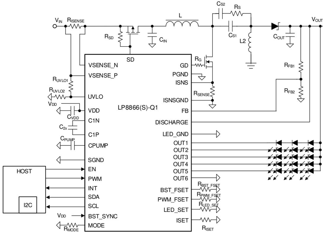
**Figure 8-7. SEPIC Mode with Three LEDs in Series**
