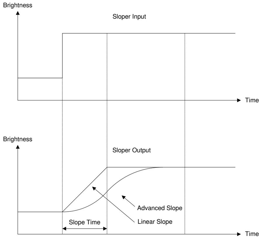
**Figure 7-13. Brightness Sloper**
