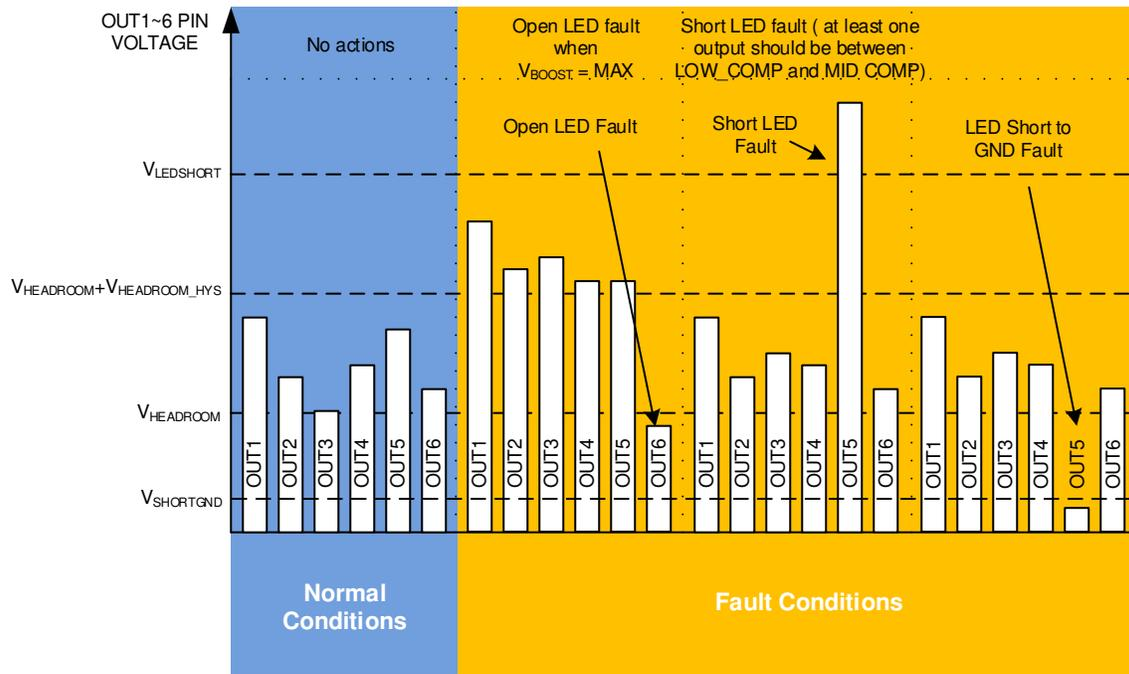
Figure 7-18. LED Open and Short Detection Logic
