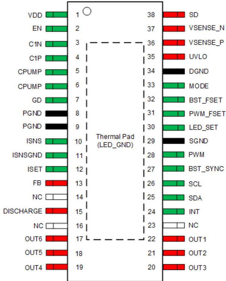
Figure 5-1. DCP Package 38-Pin HTSSOP Top View
