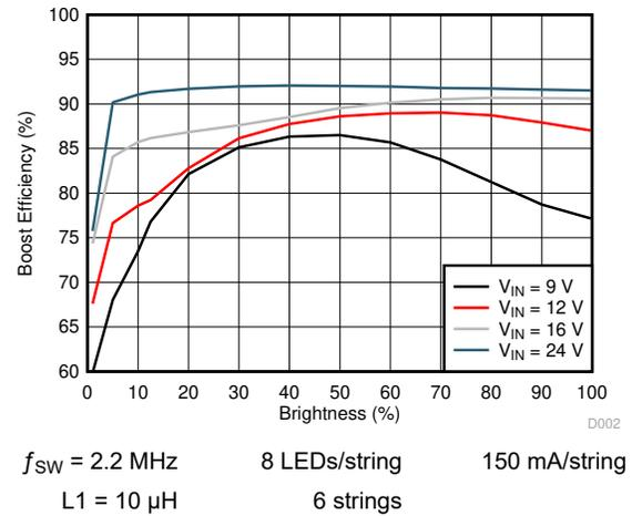
Figure 6-3. Boost Efficiency
