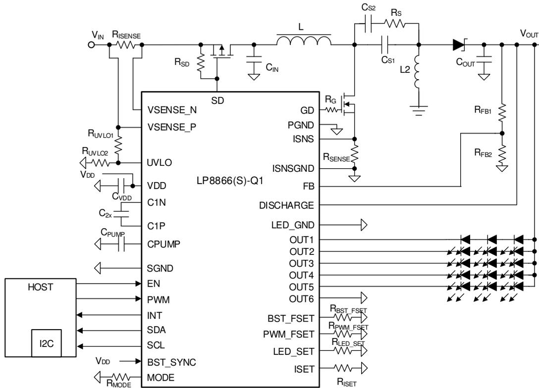
Figure 8-6. SEPIC Mode with Three LEDs in Series
