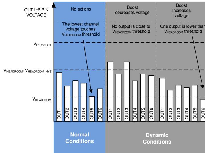
**Figure 7-4. Adaptive Boost Voltage Control Loop Function**
