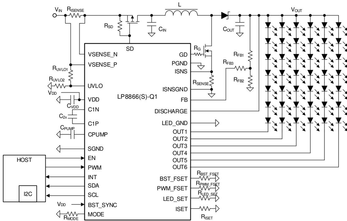
**Figure 8-2. Critical Components for Full Feature Design**
