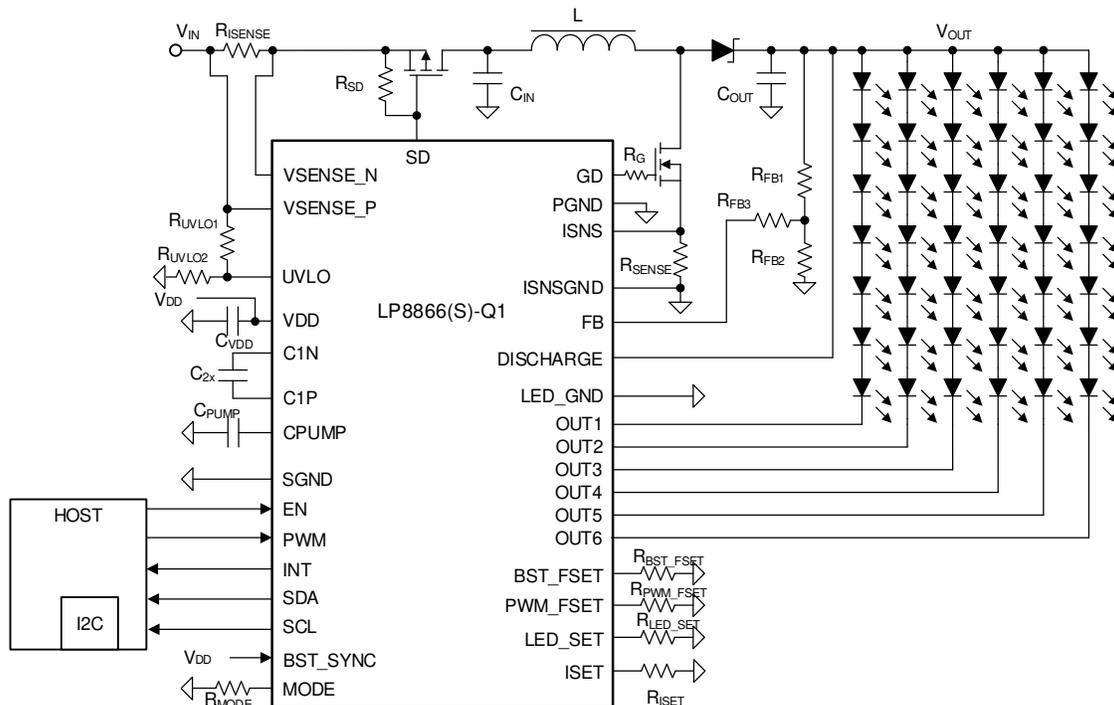
Figure 8-1. Full Feature Application for Display Backlight
