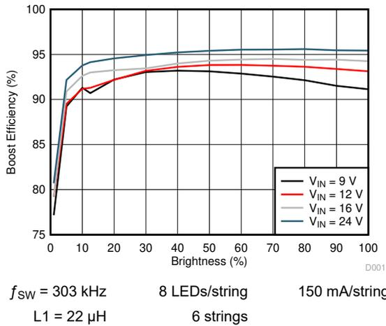
Figure 6-2. Boost Efficiency
