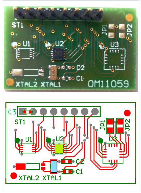
The OM11059UL allows to easily demonstrate operation of the PCF85063BTL with SPIbus interface. No need to solder the tiny package to a breadboard 100 mil connector for straight forward connections.
