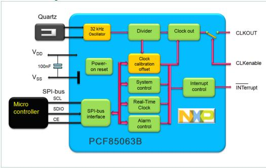
Table 2. Interfacing to microcontroller
