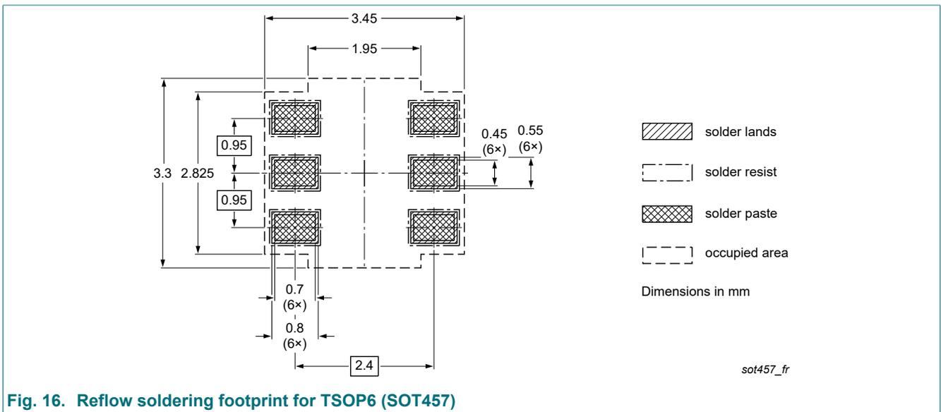
Fig. 16. Reflow soldering footprint for TSOP6 (SOT457)
