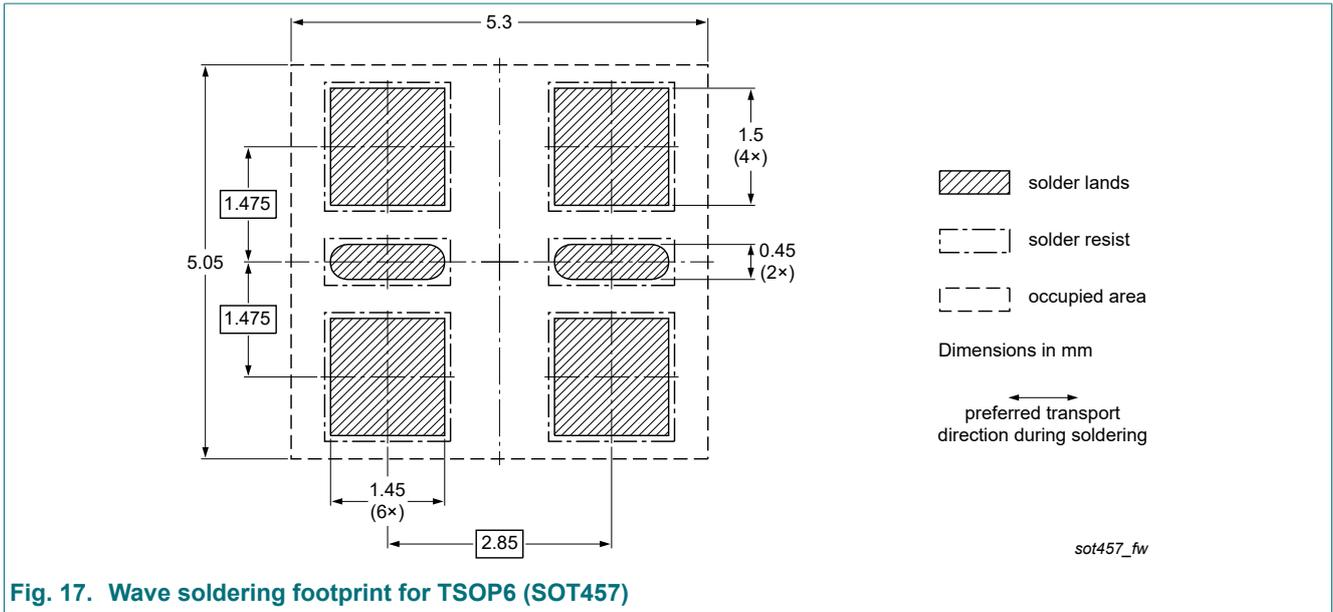
Fig. 17. Wave soldering footprint for TSOP6 (SOT457)
