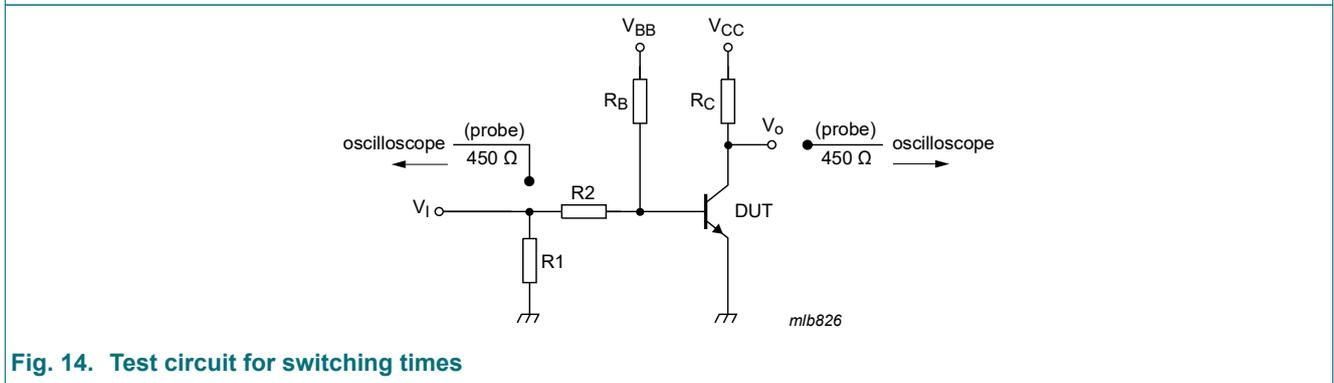
Fig. 14. Test circuit for switching times
