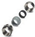
Metal screw connection up to 5 bar, thread length: 8 mm, cable diameter: 19 - 27 mm, WAF 43, screw connection: M40
