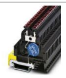
Modular terminal block with varistor as surge voltage protection between clamping connector and DIN rail, separate ground connection, nominal voltage: 60 V DC, mounting on NS 35/7.5, terminal width: 6.2 mm, terminal height: 69 mm
