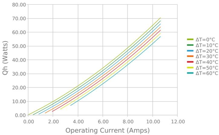
Total Heat Dissipated at Hot Side (Qh=Qc+Pin)
