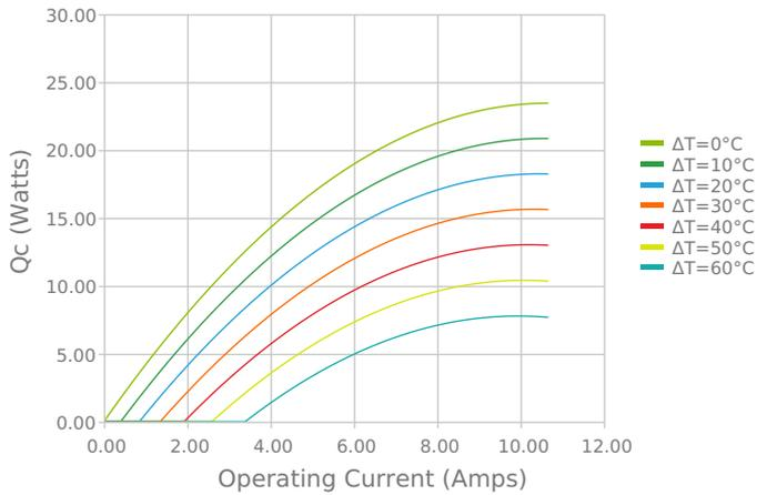
Heat Pumped at Cold Side
