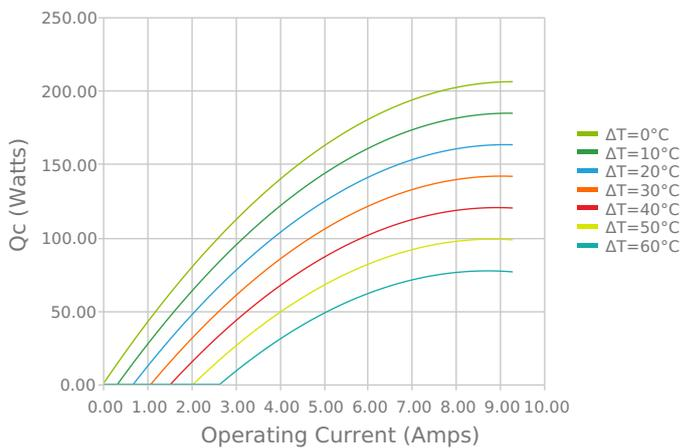
Heat Pumped at Cold Side
