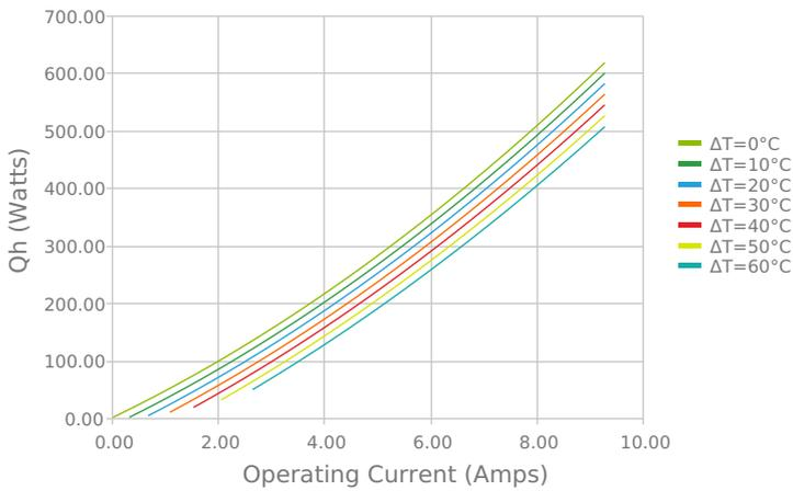
Total Heat Dissipated at Hot Side (Qh=Qc+Pin)
