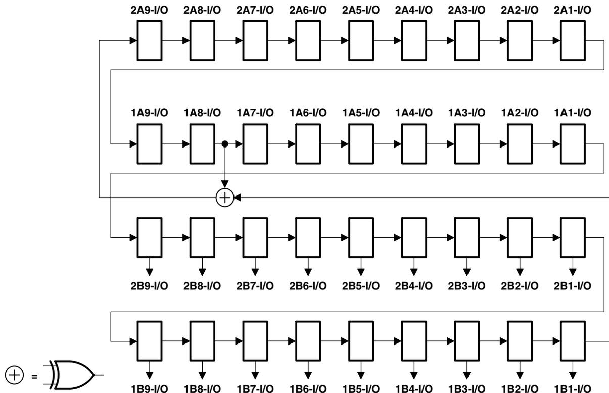
**Figure 5. 36-Bit PRPG Configuration (1OEAB = 2OEAB = 0, 1OEBA = 2OEBA = 1)**
