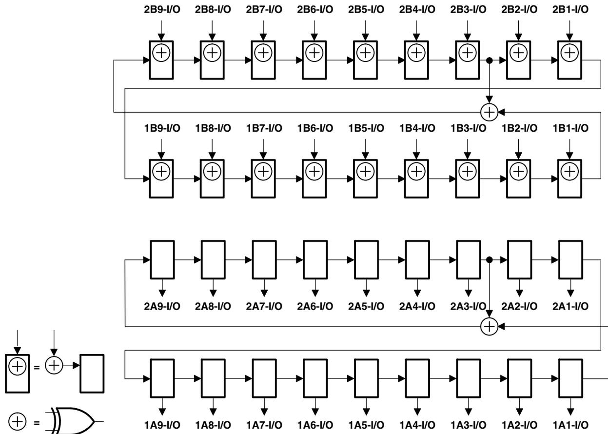
Figure 10. 18-Bit PSA/PRPG Configuration ( $1\overline{OEAB} = 2\overline{OEAB} = 1$ ,  $1\overline{OEBA} = 2\overline{OEBA} = 0$ )
