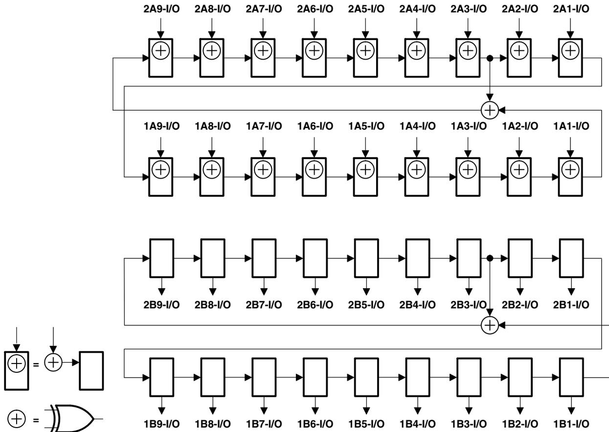
**Figure 9. 18-Bit PSA/PRPG Configuration ( $1\overline{OEAB} = 2\overline{OEAB} = 0$ ,  $1\overline{OEBA} = 2\overline{OEBA} = 1$ )**
