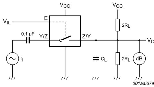
Adjust the switch input voltage for a 0 dBm level (0 dBm = 1 mW into 600  $\Omega$ ).
