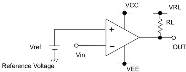
While the input voltage( $V_{in}$ ) is smaller than the reference voltage, the output voltage remains high. In case the input voltage becomes higher than the reference voltage, the output voltage will turn low.
