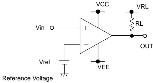
While the input voltage( $V_{in}$ ) is higher than the reference voltage, the output voltage remains high. In case the input voltage becomes lower than the reference voltage, the output voltage will turn low.
