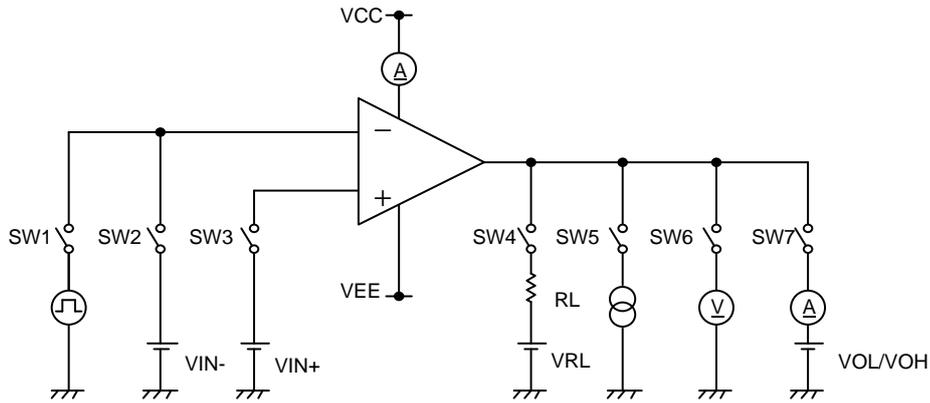
Figure 51. Test Circuit 2 (one channel only)
