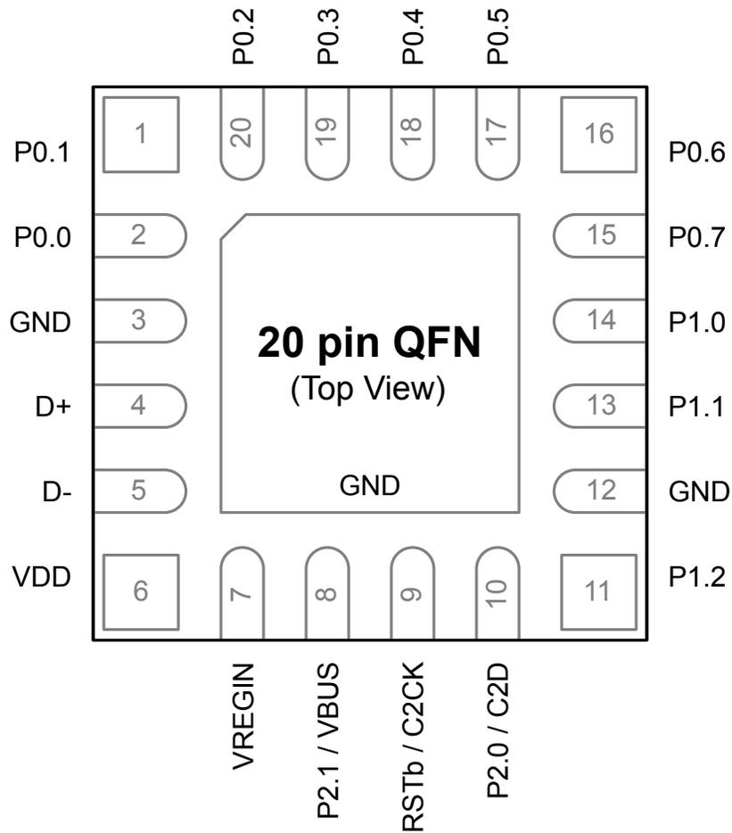
Figure 6.3. EFM8UB3x-QFN20 Pinout
