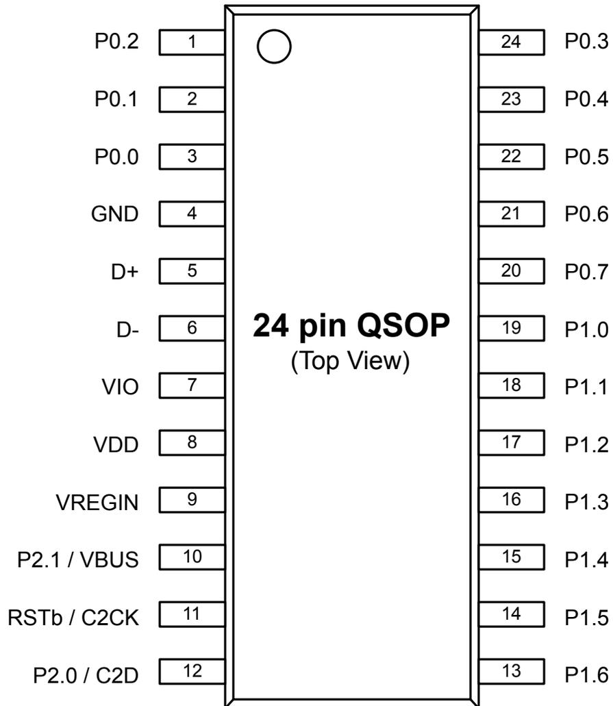
Figure 6.1. EFM8UB3x-QSOP24 Pinout
