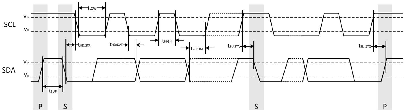
**Figure 4.1. SMBus Peripheral Timing Diagram (Master Mode)**
