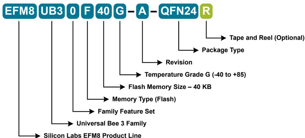
Figure 2.1. EFM8UB3 Part Numbering
