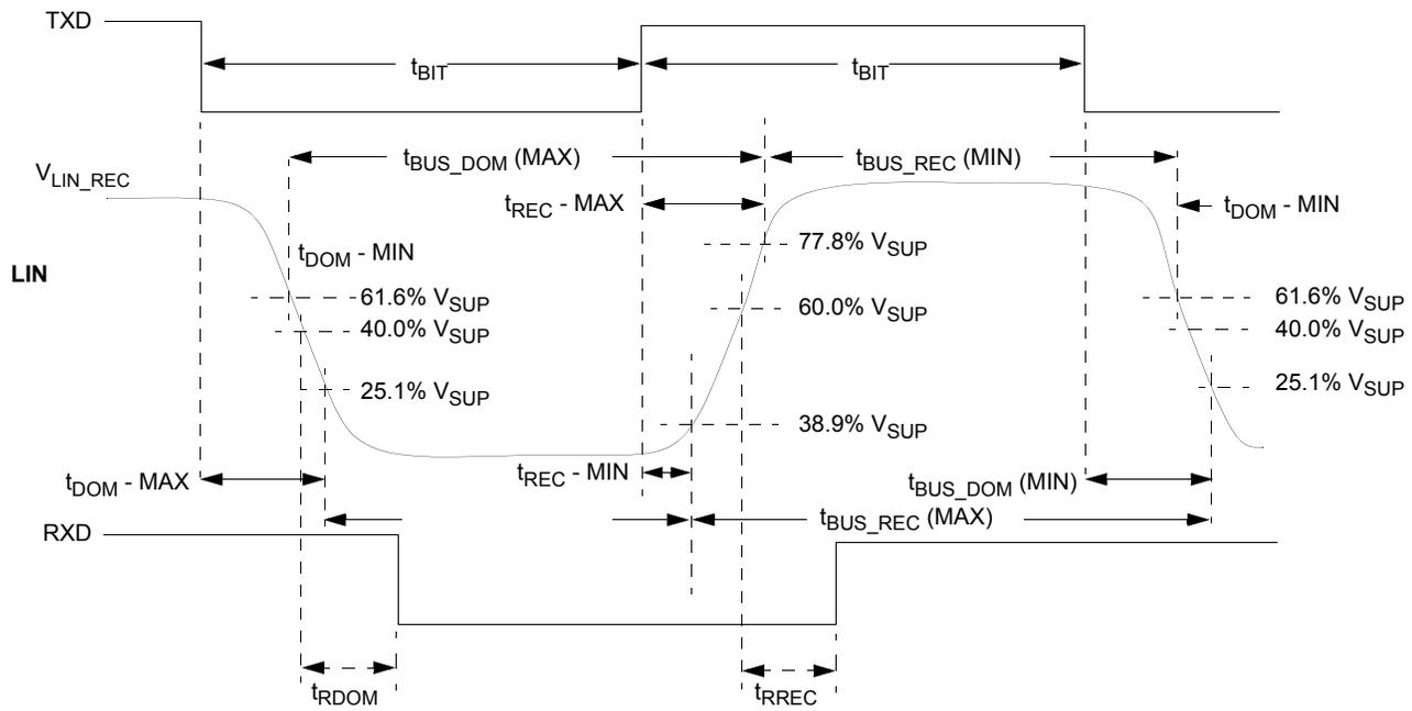
Figure 29. LIN timing measurements for slow slew rate
