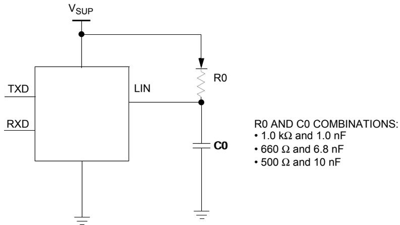
**Figure 27. Test circuit for LIN timing measurements**
