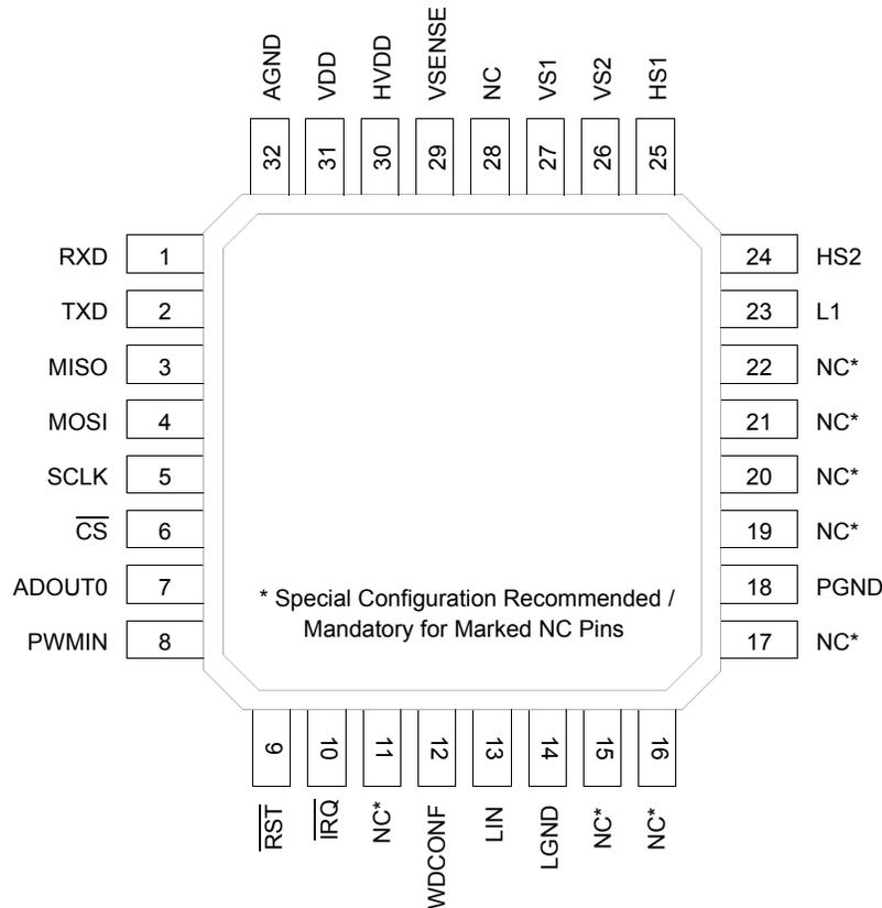
Figure 24. 33910 pin connections
