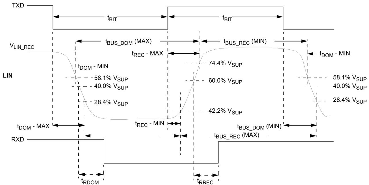
**Figure 28. LIN timing measurements for normal slew rate**
