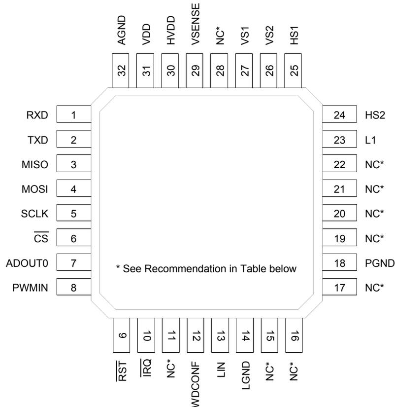
Figure 3. 33910 pin connections
