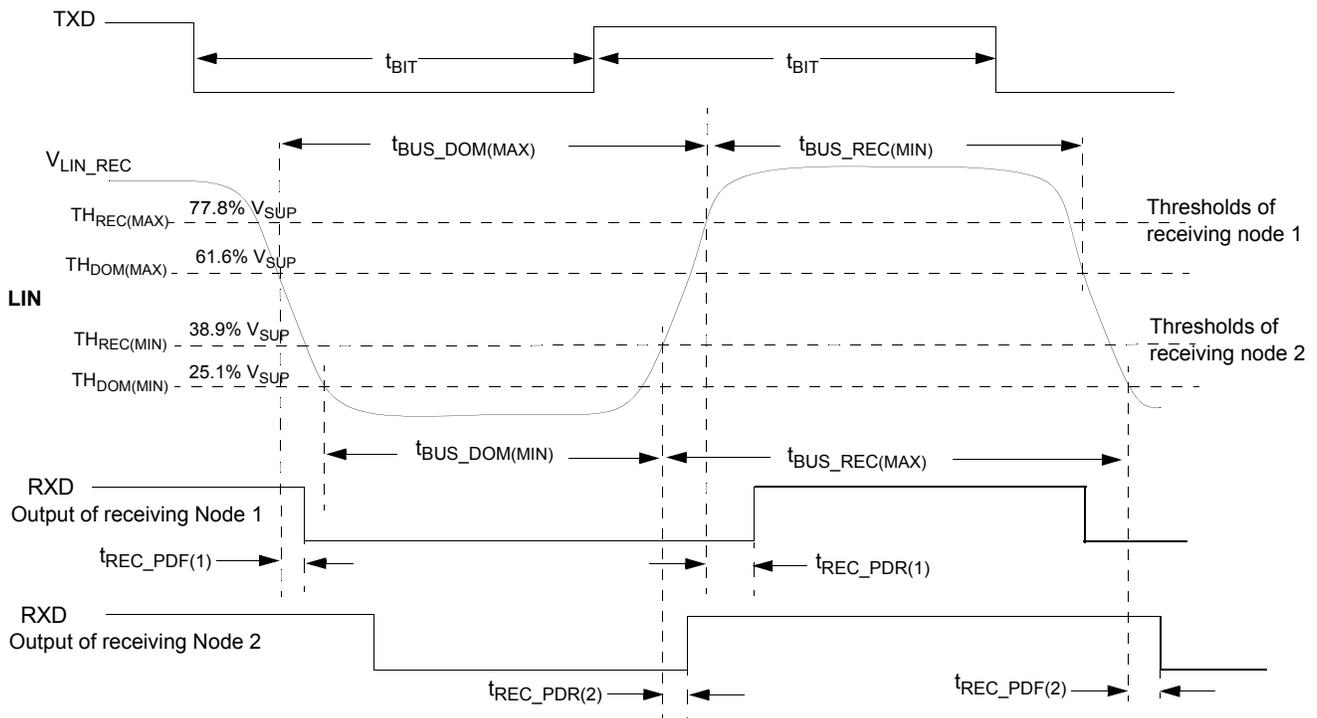
Figure 8. LIN timing measurements for slow slew rate
