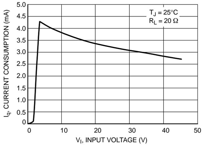
Figure 21. Current Consumption vs. Input Voltage, Adjustable Version
