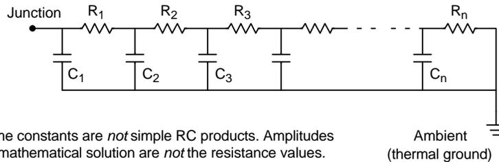
Time constants are *not* simple RC products. Amplitudes of mathematical solution are *not* the resistance values.
