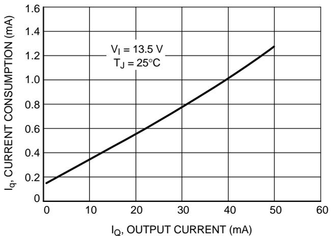
Figure 19. Current Consumption vs. Output Current (Low Load)
