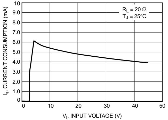
Figure 11. Current Consumption vs. Input Voltage, 3.3 V Version
