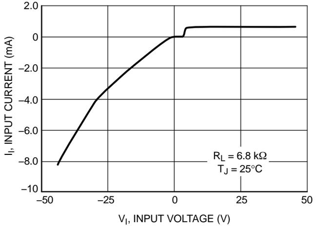
Figure 15. Input Current vs. Input Voltage, 3.3 V Version
