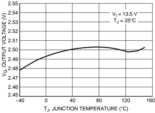
Figure 20. Output Voltage vs. Junction Temperature, Adjustable Version
