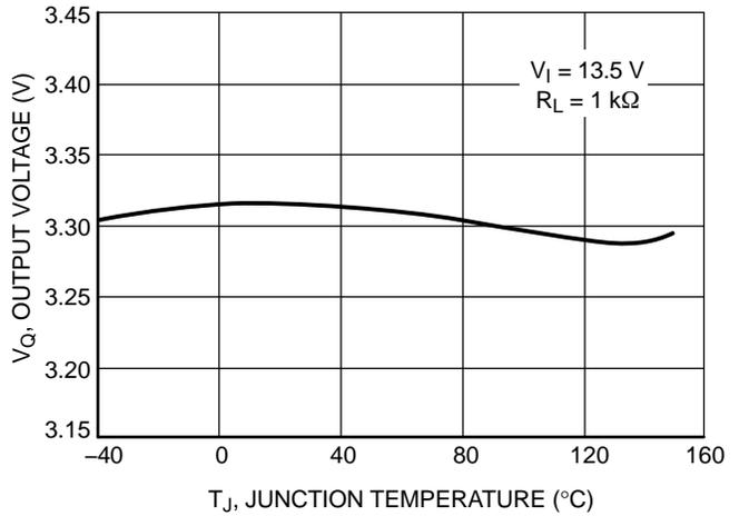
Figure 9. Output Voltage vs. Junction Temperature, 3.3 V Version
