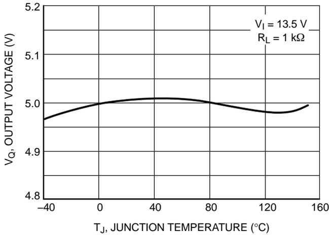
Figure 8. Output Voltage vs. Junction Temperature, 5.0 V Version
