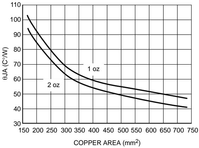
Figure 31.  $\theta_{JA}$  vs. Copper Spreader Area, DPAK 5-Lead
