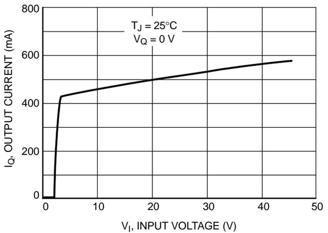
Figure 17. Maximum Output Current vs. Input Voltage
