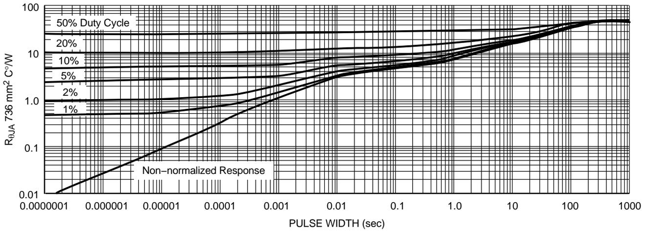
Figure 35. Duty Cycle for 1" Spread Boards, DPAK 5-Lead
