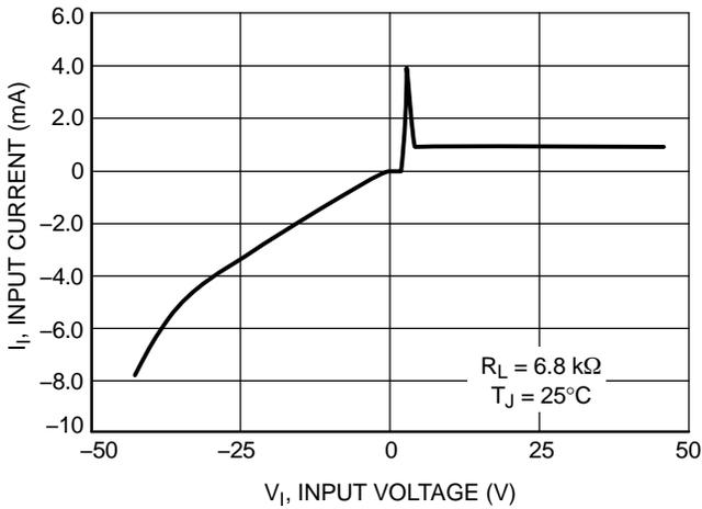
Figure 14. Input Current vs. Input Voltage, 5.0 V Version
