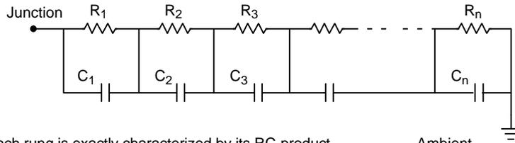
Each rung is exactly characterized by its RC-product time constant; amplitudes are the resistances.
