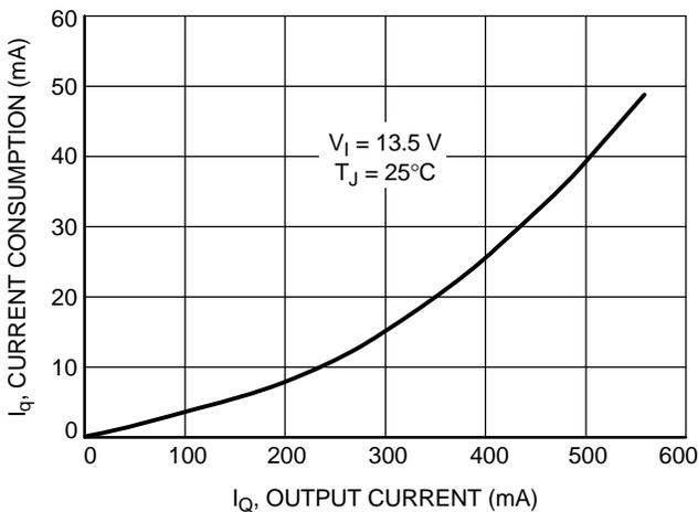
Figure 18. Current Consumption vs. Output Current (High Load)
