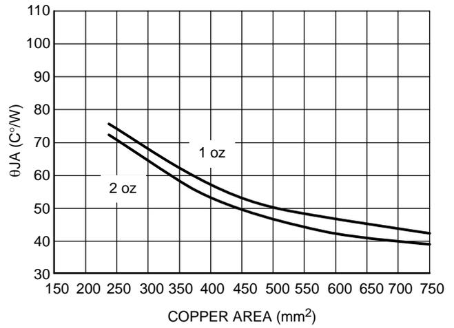
Figure 32.  $\theta_{JA}$  vs. Copper Spreader Area,  $\text{D}^2\text{PAK}$  5-Lead
