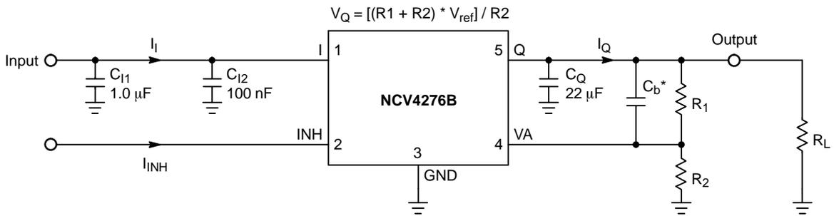
$C_b^*$  – Required if usage of low ESR output capacitor  $C_Q$  is demand, see Regulator Stability Considerations section
