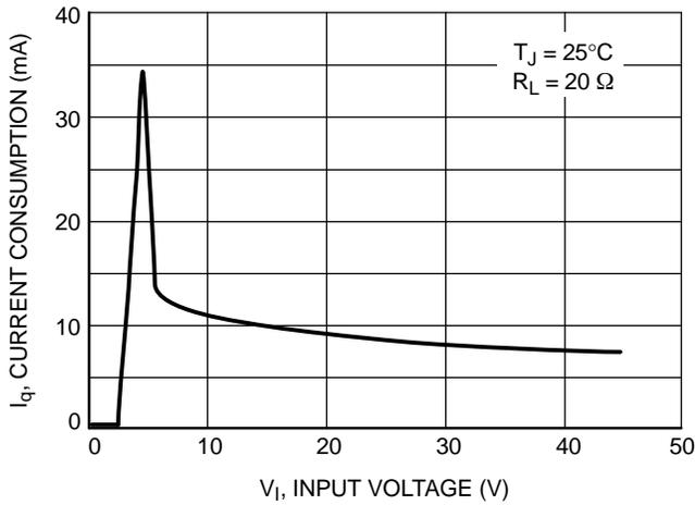
Figure 10. Current Consumption vs. Input Voltage, 5.0 V Version
