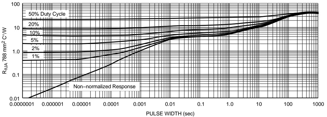
Figure 36. Duty Cycle for 1" Spread Boards, D<sup>2</sup>PAK 5-Lead
