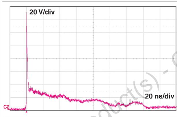
Figure 12. ESD response to IEC 61000-4-2 (-8 kV contact discharge)
