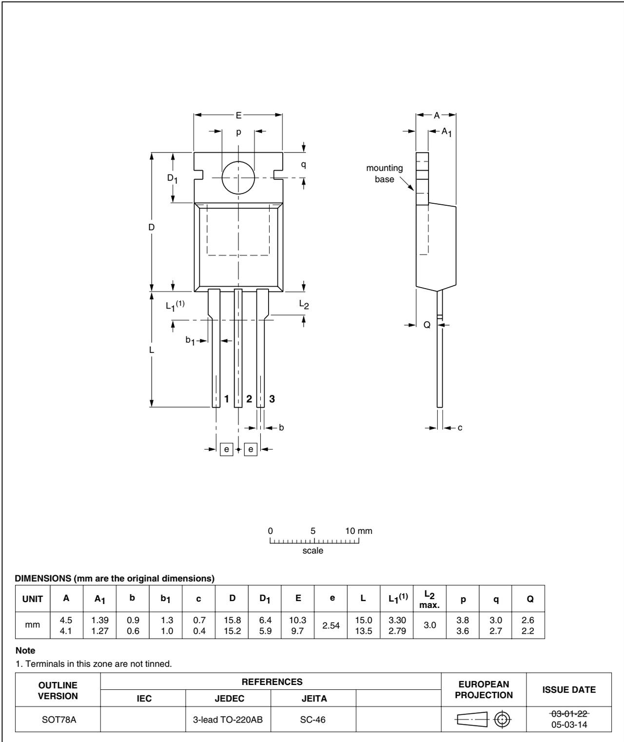
**Fig 16. Package outline SOT78A (3-lead TO-220AB; SC-46)**
