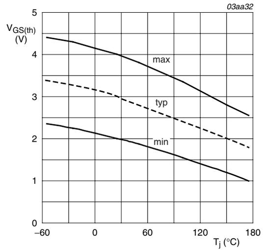
$$I_D = 1mA; V_{DS} = V_{GS}$$
