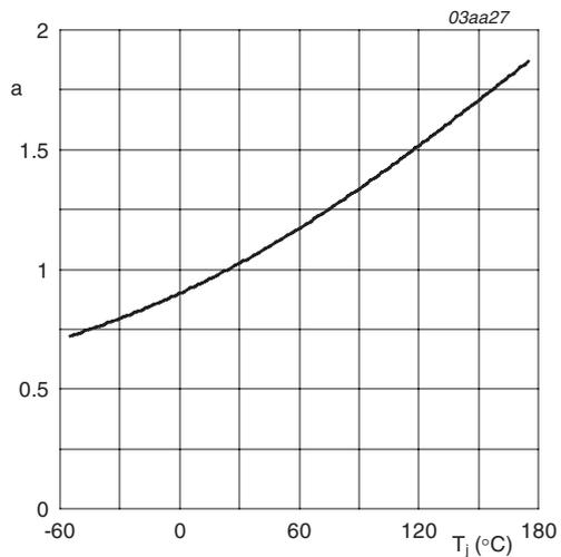
$$a = \frac{R_{DSon}}{R_{DSon(25^\circ C)}}$$
