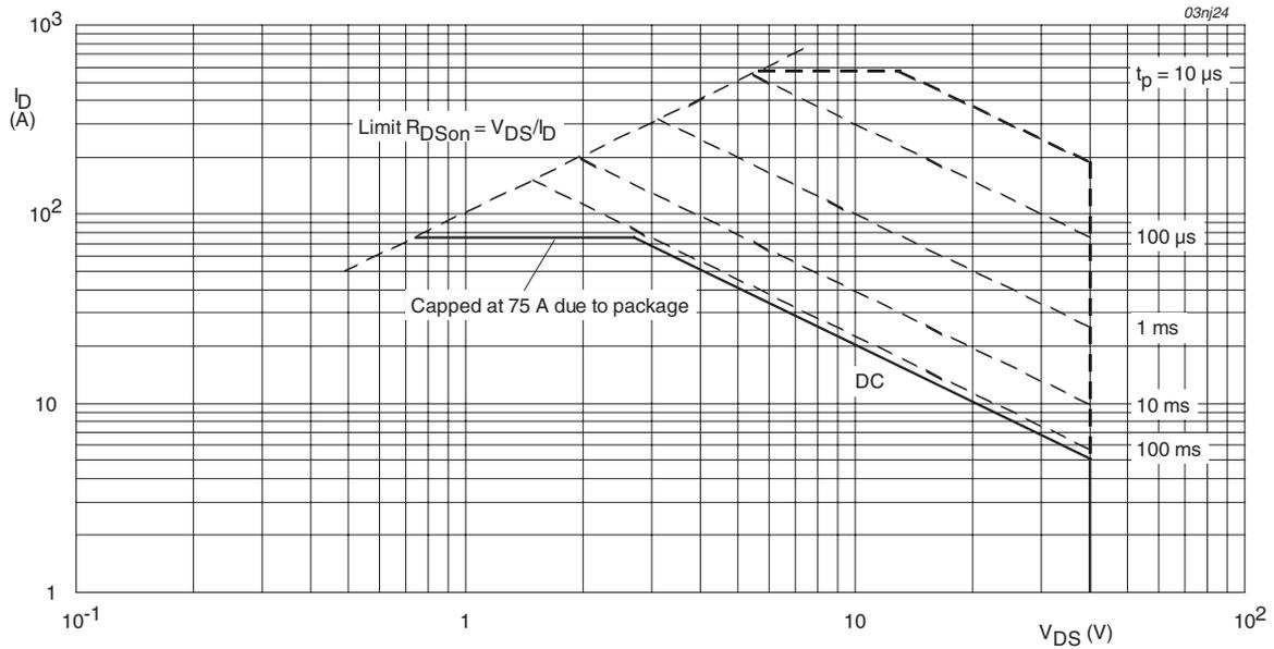
$$T_{mb} = 25^{\circ}C; I_{DM} \text{ is single pulse}$$
