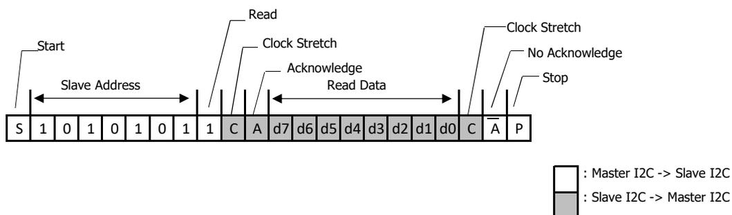
I2C read format (n byte incremental read : Device → Host)
