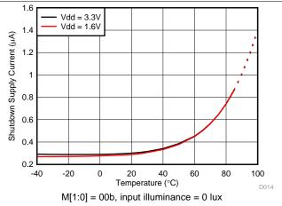
Figure 21. Shutdown Current vs Temperature (Grade 3)
