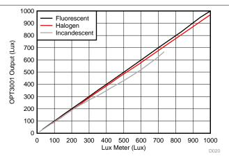
Figure 38. Compensated Output of the OPT3001-Q1 Grade 3 Device Under a Dark Window Illuminated by Fluorescent, Halogen, and Incandescent Light Sources
