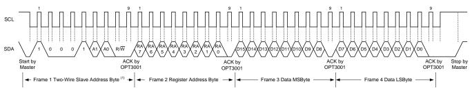
(1) The value of the slave address byte is determined by the setting of the ADDR pin; see Table 1.
