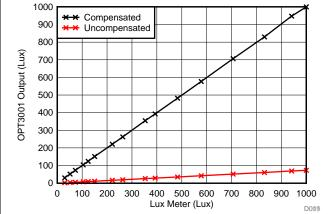
Figure 37. Uncompensated and Compensated Output of the OPT3001-Q1 Grade 3 Device Under a Dark Window Illuminated by Fluorescent Light Source
