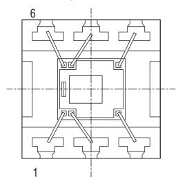
Figure 40. Package Orientation Visual Reference of Pin 1 (Top View)
