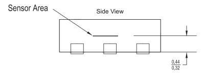
Figure 41. Mechanical Outline Showing Sensing Area Location (Top and Side Views)
