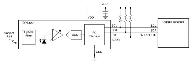
Figure 33. Measuring Ambient Light in a Product Case Behind a Dark Window
