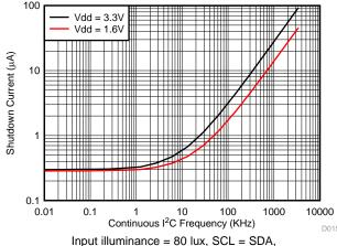
continuously toggled at I<sup>2</sup>C frequency
