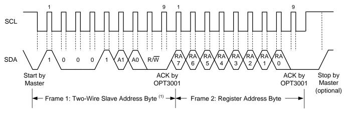
(1) The value of the slave address byte is determined by the ADDR pin setting; see Table 1.
