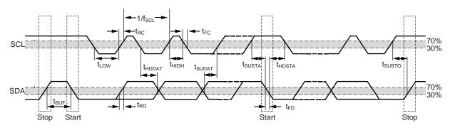
Figure 1. I<sup>2</sup>C Detailed Timing Diagram
