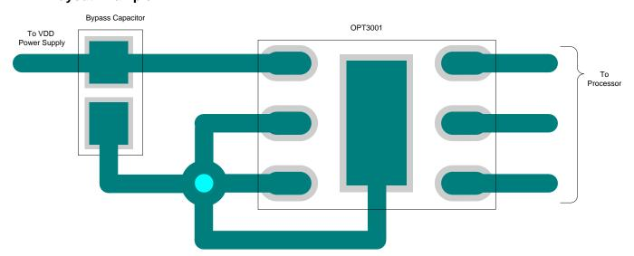
Figure 39. Example PCB Layout With the OPT3001-Q1 Device
