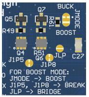
Figure 5: Power configuration jumpers (Default)
