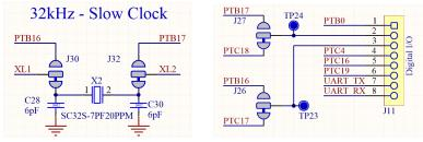
Figure 16: Schematic: 32 kHz oscillator
