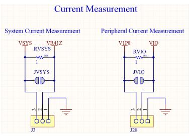
Figure 7: Schematic: Current measurement headers
