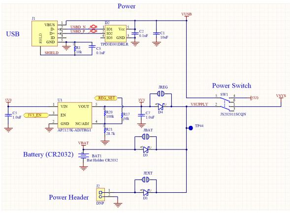
Figure 3: Schematic: Power supply
