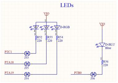
Figure 11: Schematic: User LEDs
