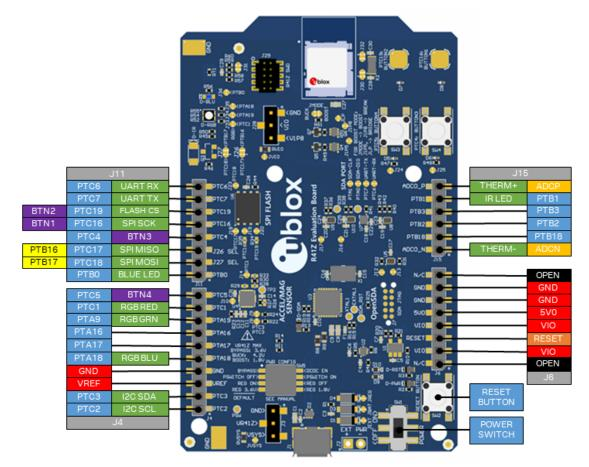
Figure 9: Expansion header pinout
