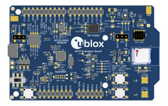
Figure 1: EVK-R41Z evaluation board (Top view)
