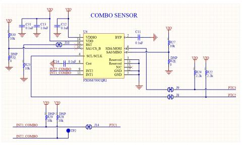
Figure 15: Schematic: I2C combo sensor
