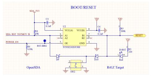
Figure 8: Schematic: Reset button
