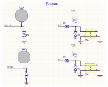
Figure 13: Schematic: User buttons
