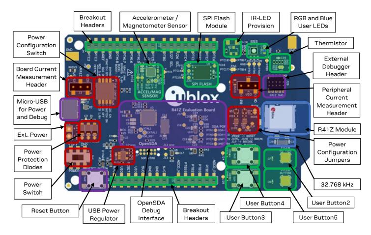
Figure 2: Evaluation board layout
