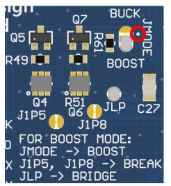
Figure 6: Power configuration jumpers (Boost mode)
