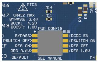
Figure 4: Power configuration switch
