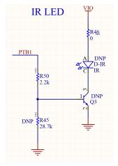
Figure 10: Schematic: IR LED
