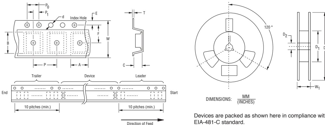
Devices are packed as shown here in compliance with EIA-481-C standard.
