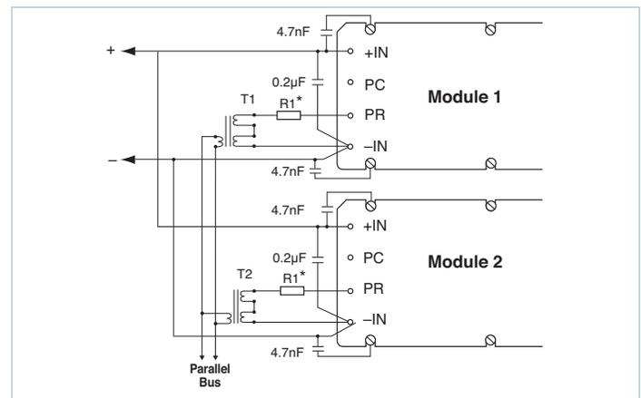
Figure 10 — Transformer-coupled interface
