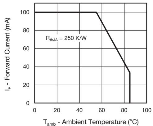
Fig. 2 - Forward Current Limit vs. Ambient Temperature
