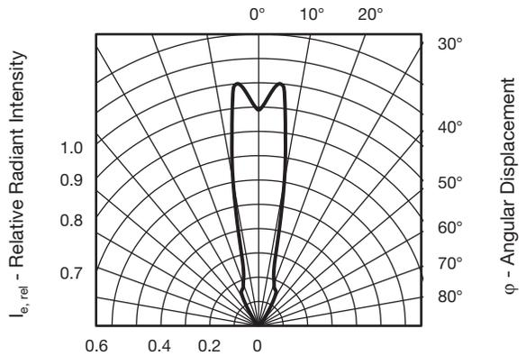
Fig. 8 - Relative Radiant Intensity vs. Angular Displacement
