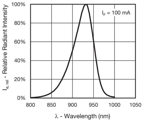
Fig. 7 - Relative Radiant Intensity vs. Wavelength
