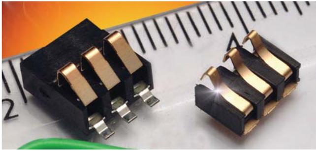
The newest product in KYOCERA AVX Interconnect family of battery connectors saves 50% in volume over the initial 9155 series compression connectors as illustrated in the photograph. These connectors are rated at a full 3 amps per contact on 2.5mm centers. Sizes range from 2 positions through 5 positions and are end to end stackable.
