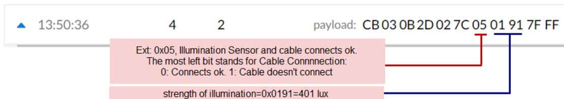
**Means:** The device is set to connect to an Illumination sensor, the cable connection is **fine**. This strength of illumination is 401 lux
