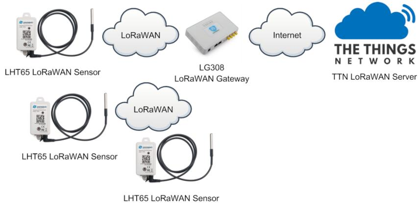
Assume the LG308 is already set to connect to [TTN V3 network](#). We need to add the LHT65 device in TTN V3:
