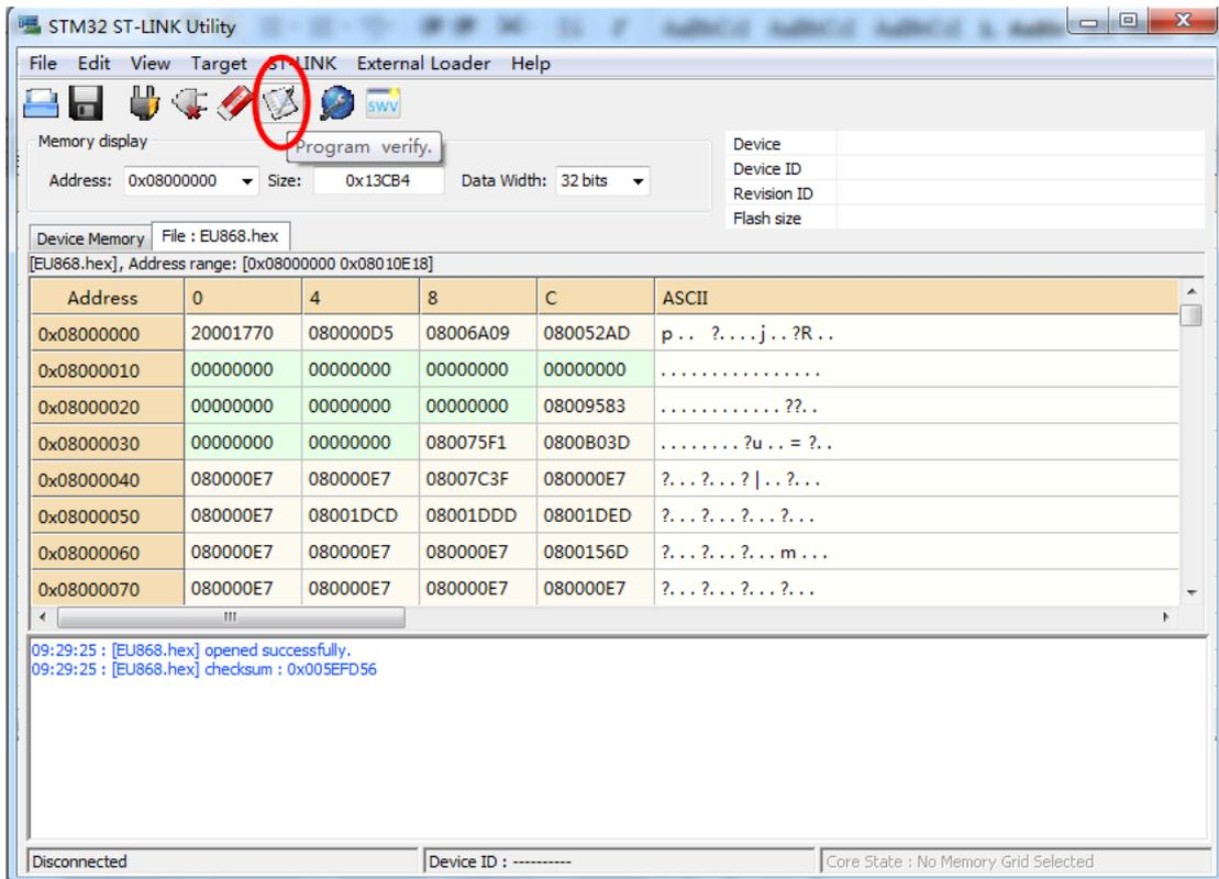
**Step5:** The led on the ST-LINK adapter will now blinking, click program verify button to select the image to be upgraded.
