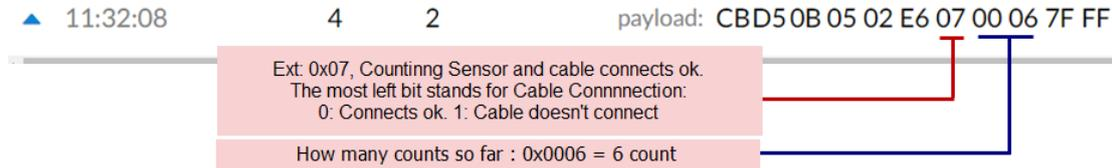
**Means:** The device is set to connect to a counting sensor, the cable connection is **fine**. It detects 6 times event so far.
