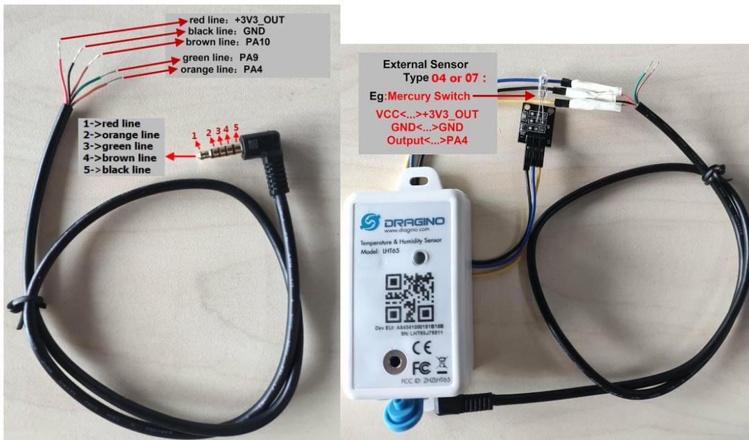
Above is connection to a mercury switch, rotate the mercury will generate interrupt. LHT65 will count it. It will periodically the counting value to server. User can also connect PA9 and PA10 together, with these two pins shortcut, LHT65 will know if the probe is connected well in the socket.
