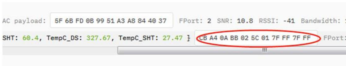
Check the battery voltage for LHT65.
