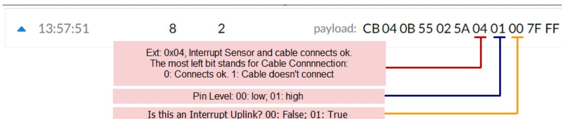
**Means:** The device is set to connect to an Interrupt Sensor, the cable connection is **fine**. This packet is for a **normal uplink**, pin level is **high**.
