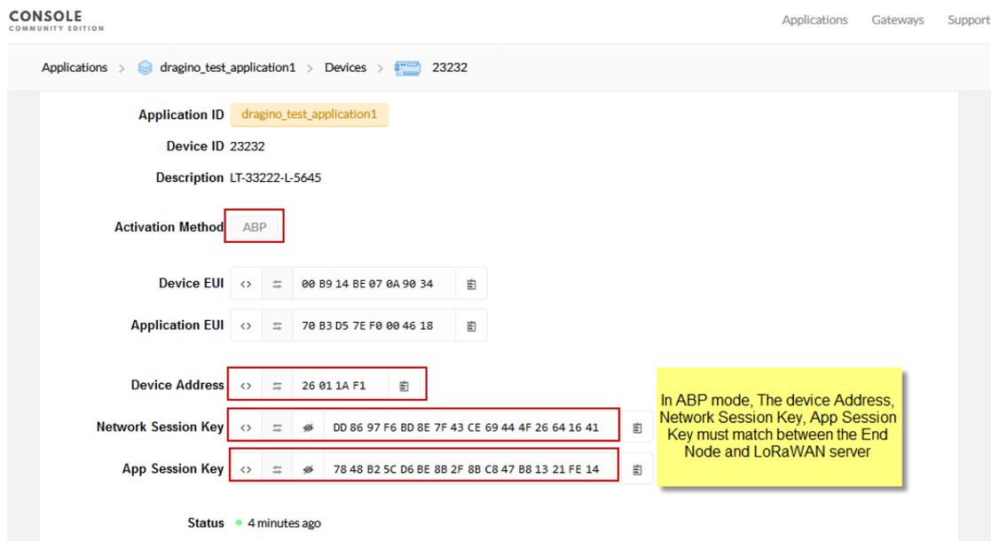
**Note:** user just need to make sure above three keys match, User can change either in TTN V3 or Device to make then match. In TTN V3, NETSKEY and APPSKEY can be configured by user in setting page, but Device Addr is generated by TTN V3.
