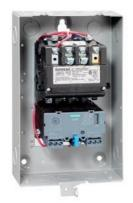
Non-reversing motor starter, Size 1, Three phase full voltage, Solid-state overload relay, OLR amp range 10-40A, 208VAC 60Hz coil, Non-combination type, Enclosure type 1, Indoor general purpose use, Standard width enclosure
