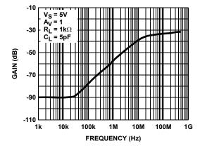
FIGURE 15. DISABLED OUTPUT ISOLATION FREQUENCY **RESPONSE**
