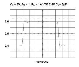
FIGURE 21. SMALL SIGNAL TRANSIENT RESPONSE
