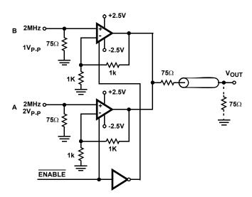
FIGURE 29. TWO TO ONE MULTIPLEXER
