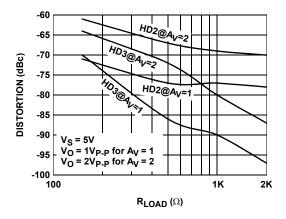
FIGURE 17. HARMONIC DISTORTION vs LOAD RESISTANCE
