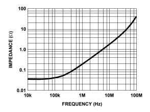
FIGURE 11. OUTPUT IMPEDANCE vs FREQUENCY
