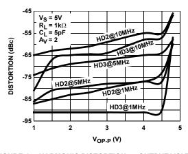
FIGURE 14. HARMONIC DISTORTION vs OUTPUT VOLTAGE
