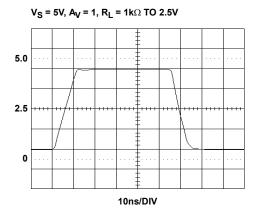
FIGURE 19. LARGE SIGNAL TRANSIENT RESPONSE
