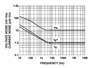
FIGURE 18. VOLTAGE AND CURRENT NOISE vs FREQUENCY
