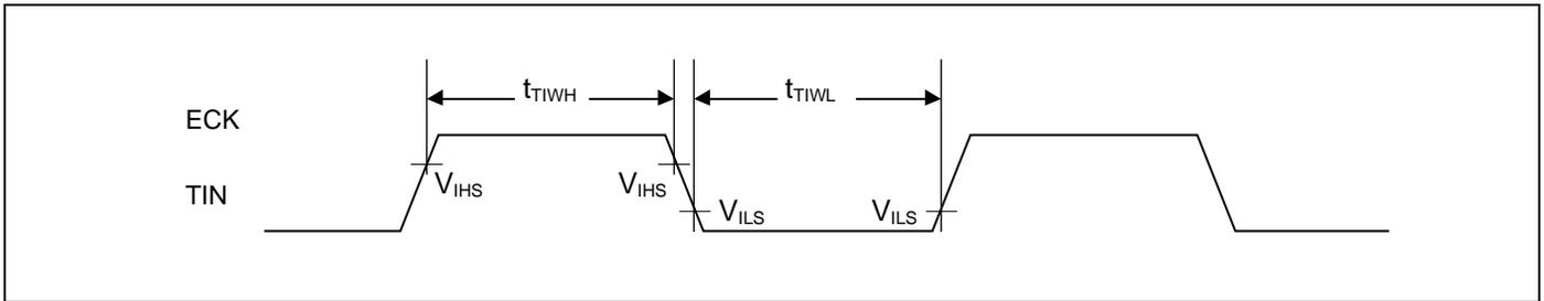
**Trigger input timing**
