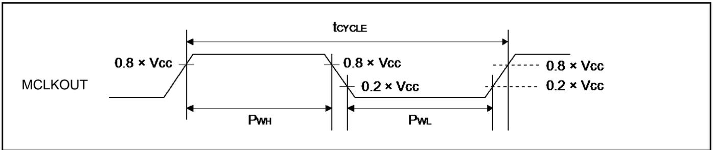
**External bus signal input/output characteristics**
