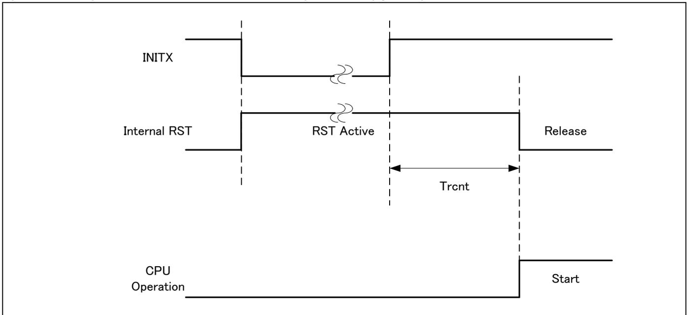
**Operation example of return from low power consumption mode (by internal resource reset<sup>[1]</sup>)**
