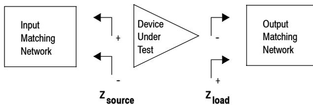
Figure 14. Series Equivalent Source and Load Impedance
