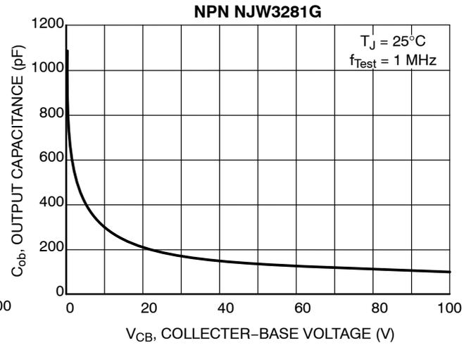
**Figure 14. Output Capacitance**
