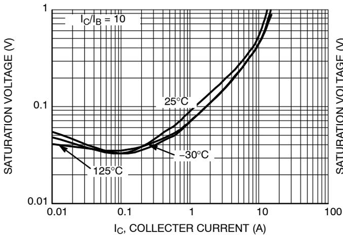
Figure 9.  $V_{CE(sat)}$ , Collector-Emitter Saturation Voltage
