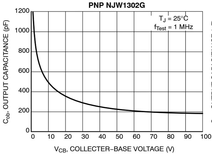
**Figure 13. Output Capacitance**
