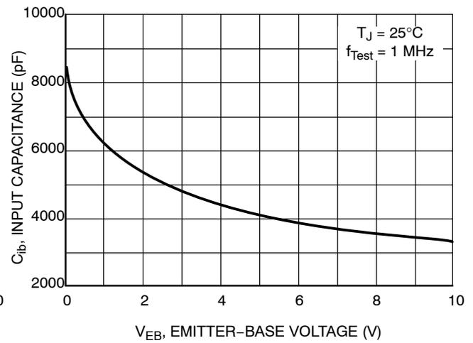
**Figure 16. Input Capacitance**
