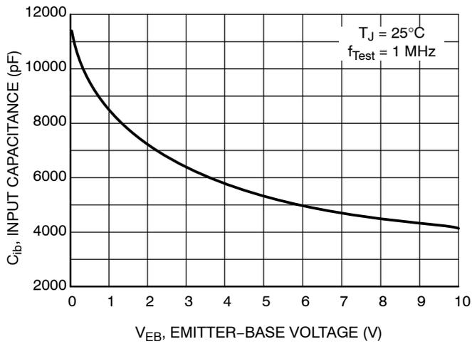
**Figure 15. Input Capacitance**
