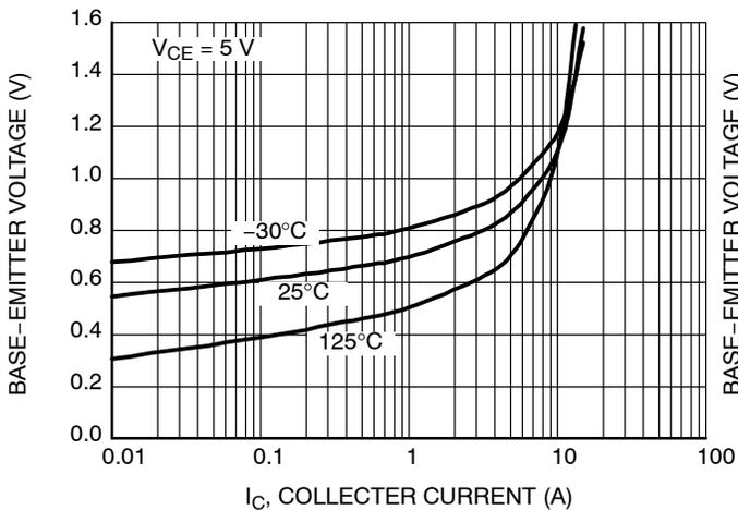
Figure 11.  $V_{BE(on)}$ , Base-Emitter Voltage
