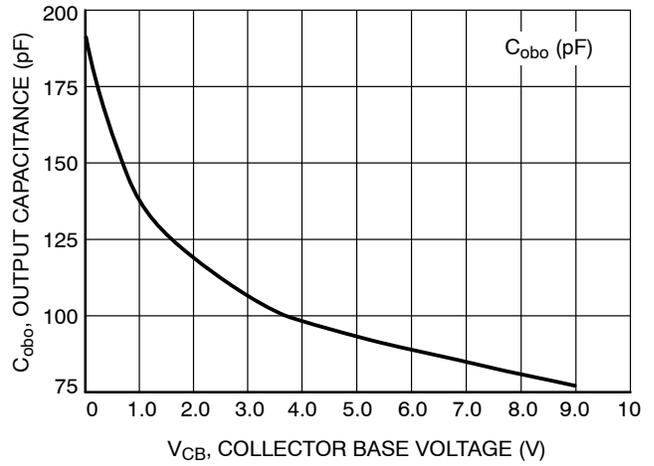
Figure 8. Output Capacitance
