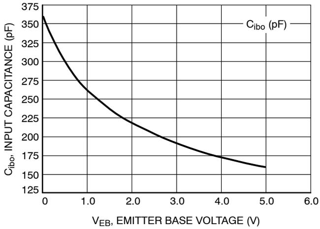
Figure 7. Input Capacitance
