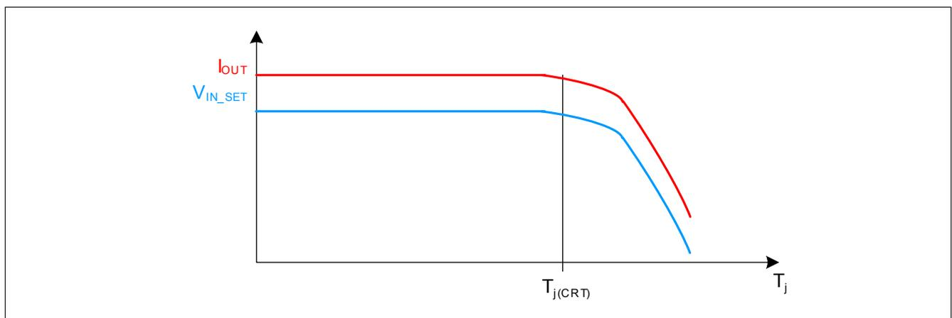
**Figure 20** Output current reduction at high temperature
