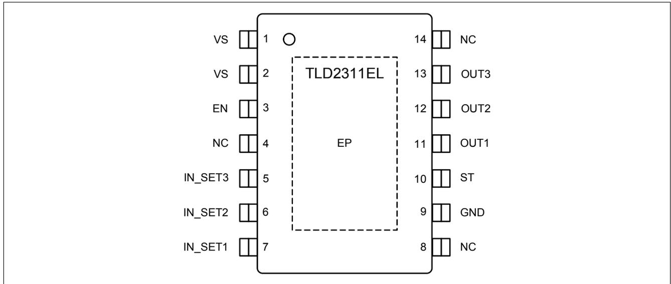
Figure 2 Pin Configuration
