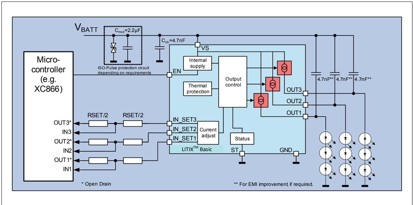
Figure 21 Application Diagram with Diagnosis for each channel
