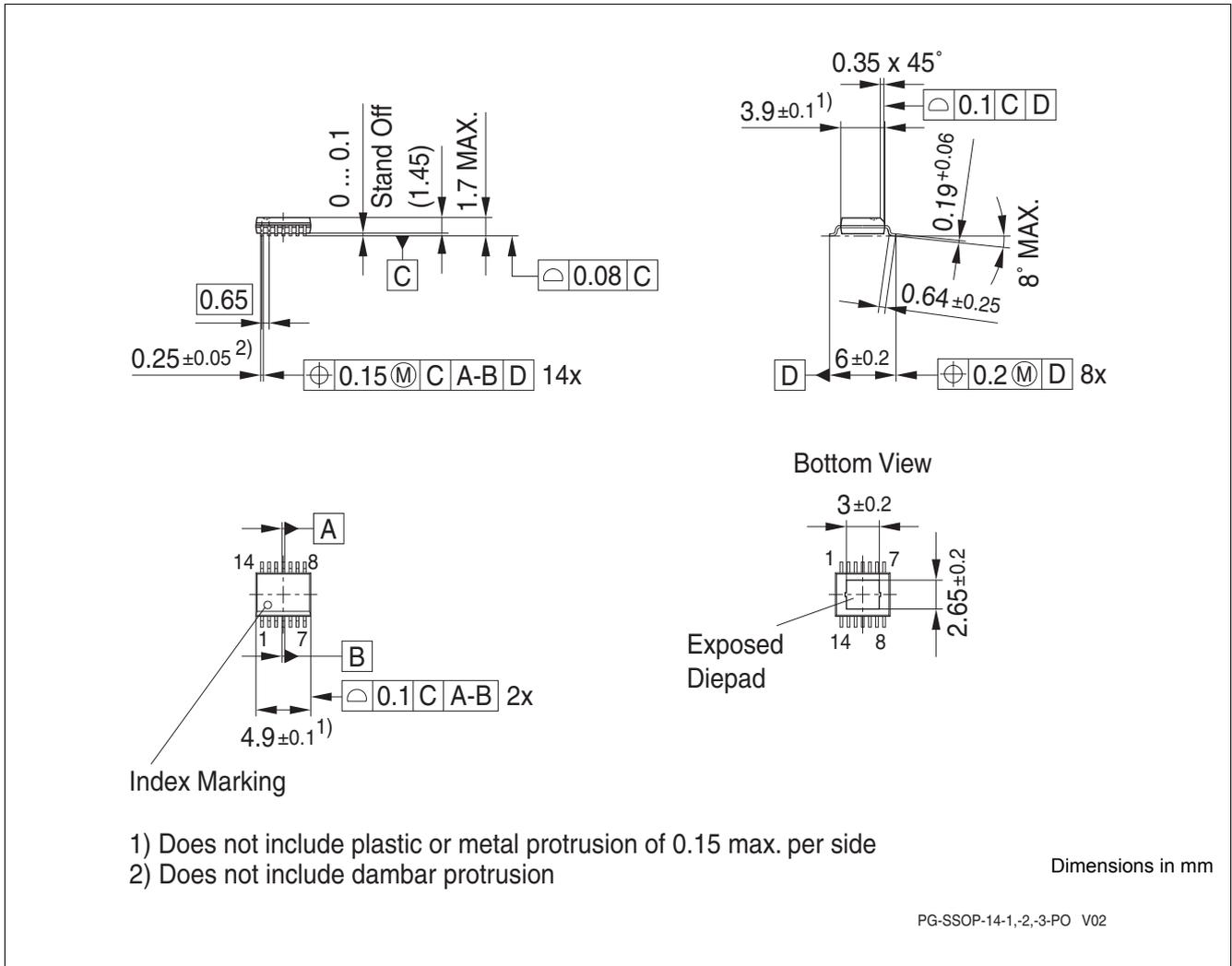
Figure 22 PG-SSOP14
