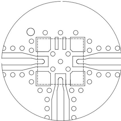
DXF available on request based on 10 mil RO4350 substrate.
