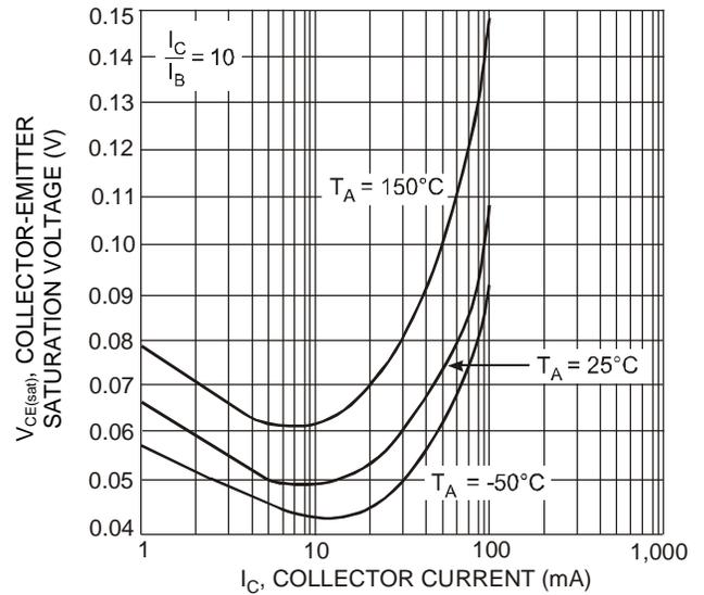
**Figure 6. Typical Collector-Emitter Saturation Voltage vs. Collector Current**
