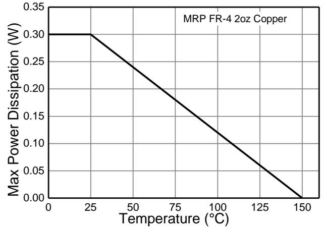
**Figure 2. Derating Curve**
