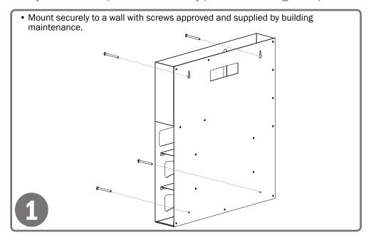
• Dispenser can be mounted onto a BOWMAN® door or wall hanger through the cutout in the back.
