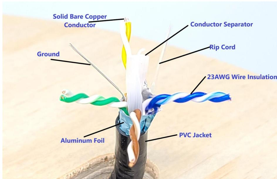
Our cable allows for maximum performance while minimizing electromagnetic interference/radio-frequency interference (EMI/RFI) and almost eliminating alien crosstalk (AXT).
