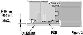
There should be no broken stand-offs along the perimeter of the part (an indication of over-pressing).
