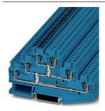
Multi-level terminal block, With equipotential bonder, nom. voltage: 500 V, nominal current: 20 A, connection method: Spring-cage connection, number of connections: 6, cross section: 0.08 mm² - 4 mm², AWG: 28 - 12, width: 5.2 mm, color: blue, mounting type: NS 35/7,5, NS 35/15
