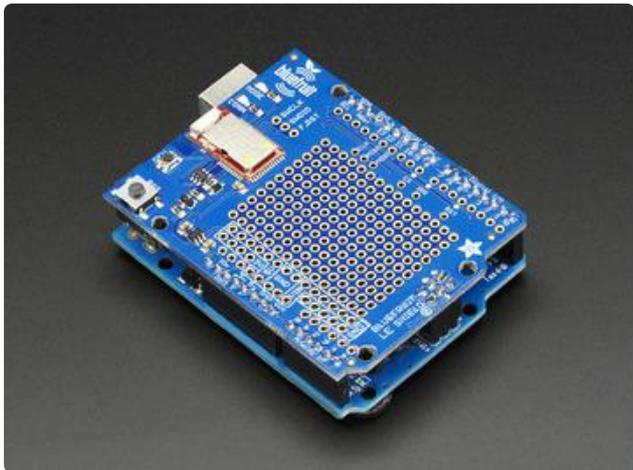
If you are using the Bluefruit LE Shield then you have an SPI-connected NRF51822 module. You can use this with Atmega328 (Arduino UNO or compatible), ATmega32u4 (Arduino Leonardo, compatible) or ATSAM21 (Arduino Zero, compatible) and possibly others. Your pinouts are Hardware SPI, CS = 8, IRQ = 7, RST = 4
