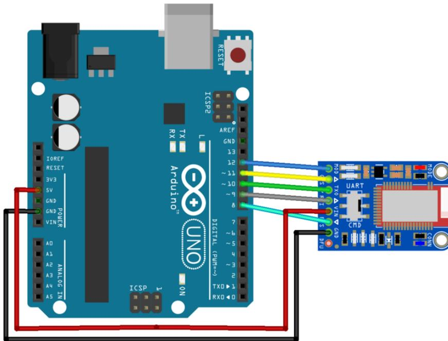
All of these pins are 'flexible' and you can change them around as necessary after you get your setup running nicely, but we recommend starting out with our default wiring.
