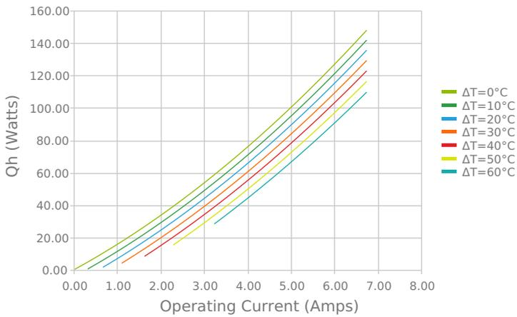
Total Heat Dissipated at Hot Side (Qh=Qc+Pin)
