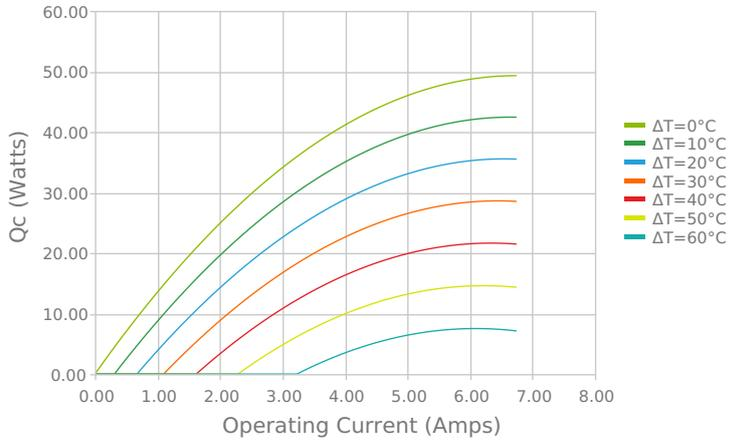
Heat Pumped at Cold Side
