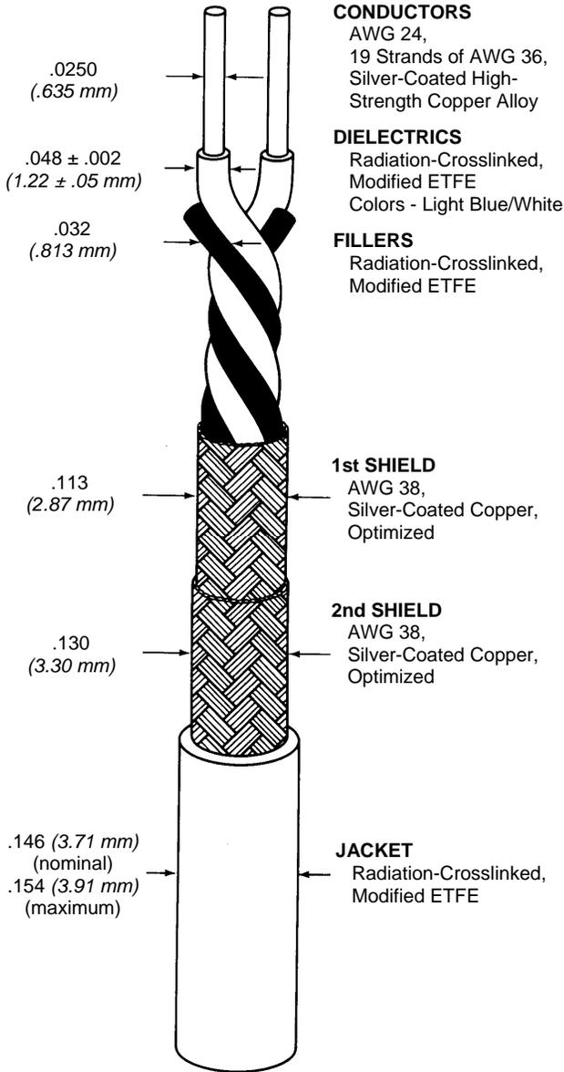
Designate outer jacket color with a dash number in accordance with MIL-STD-681. Unless otherwise specified, outer jacket color will be white designated by a "-9" appended to the part number, (e.g. 7724G3664-9). Other codes and suffixes may be added to the part number, as necessary, to capture any additional requirements imposed by the purchase order.
