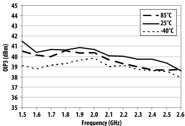
Figure 24. OIP3 over Frequency and Temperature
