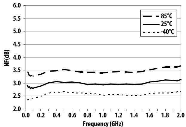
Figure 13. Noise Figure over Frequency and Temperature
