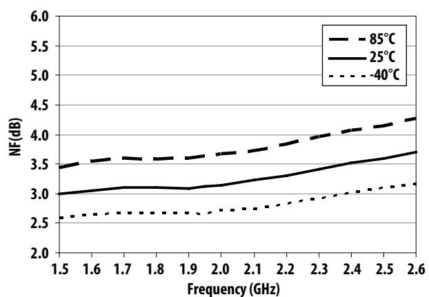
Figure 29. Noise Figure over Frequency and Temperature
