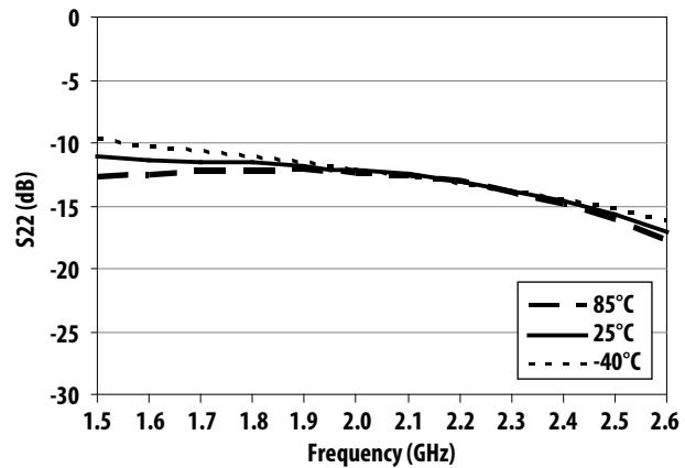
Figure 27. S22 over Frequency and Temperature
