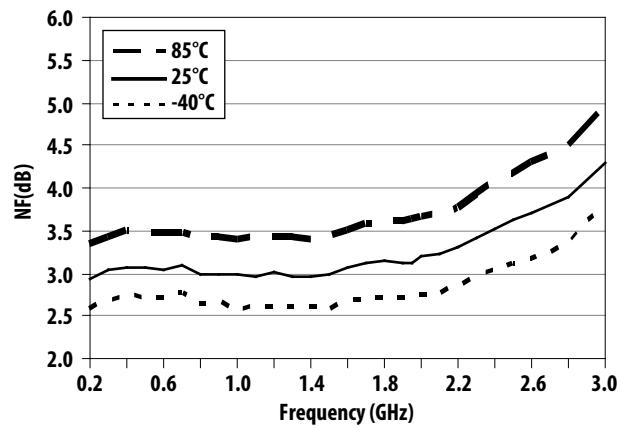
Figure 21. Noise Figure over Frequency and Temperature
